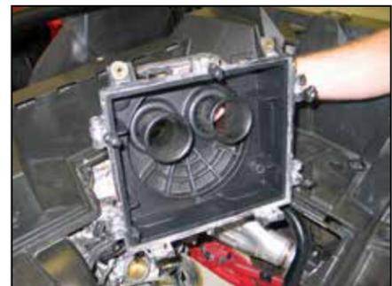
9. Remove the air box half from the vehicle as shown.
