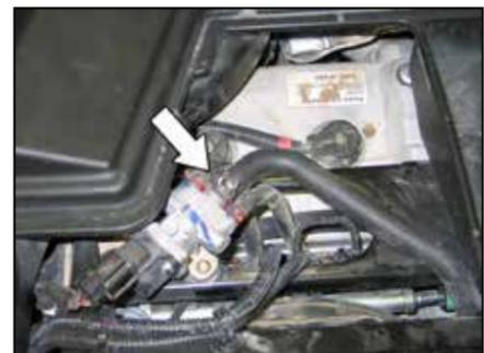
8. Loosen the hose clamp that secures the idle by-pass hose to the idle by-pass solenoid.
