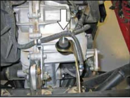
12. Install the rubber mounted stud onto the heat shield mount as shown.
