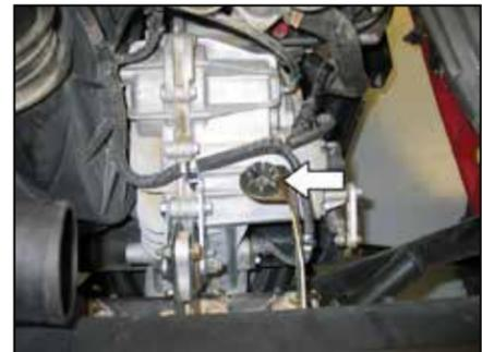
10. Remove the lower air box mounting grommet shown.
