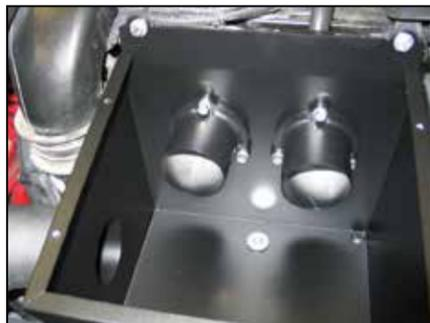
20. Install the left side intake tube (27548) through the heat shield and into the silicone hose on the throttle body, and then secure with the provided hardware and hose clamp.
