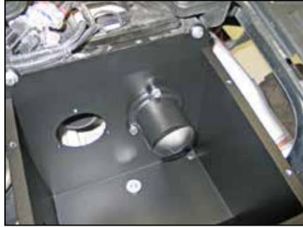
17. Install the right side intake tube (27547) through the heat shield, rotate 180° and then install into the silicone hose at the throttle body. Secure the intake tube with the hose clamp and hardware provided.
