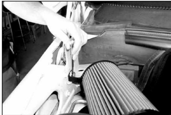
17. Attach the filter bracket to inner fender using the bolt removed in step 15.
