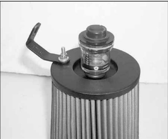
14. Install the grommet and restriction gauge into the hole in the top plate of the air filter.
