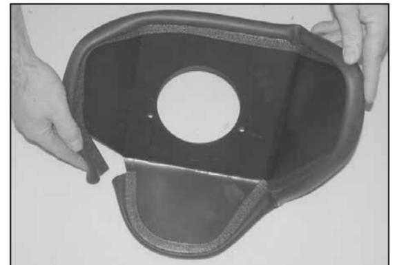
9. Install the provided edge trim onto the heat shield as shown.
