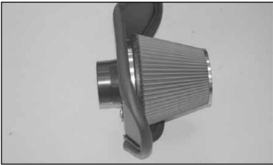
11. Install the K&N® air filter onto the filter adapter as shown.
