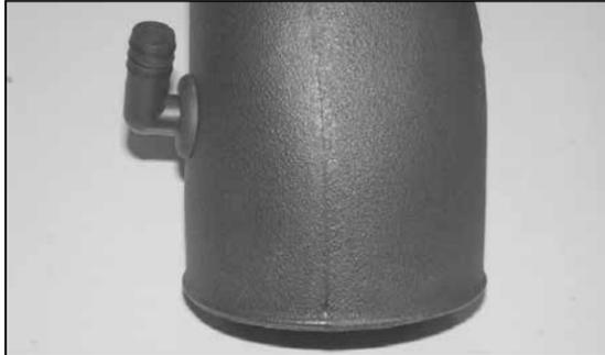
17. Install the provided elbow fitting into the grommet installed in step #16 as shown.
