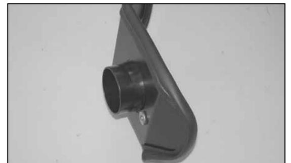
10. Install the air filter adapter onto the heat shield with the provided hardware.
