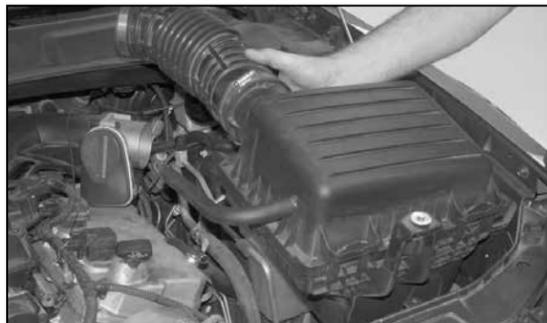
6. Lift the complete intake and air filter assembly to remove it from the vehicle.
