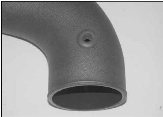
16. Install 2nd supplied grommet into the filter end of the K&N® intake tube as shown.
