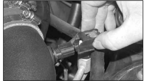
22. Reconnect the air temperature electrical connection as shown.
