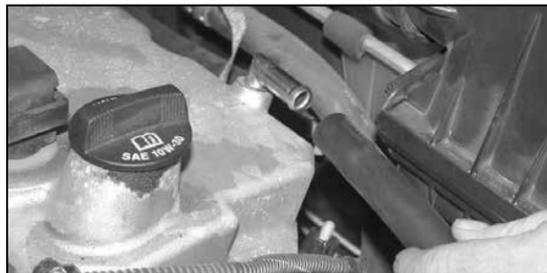
4. Disconnect the crankcase vent hose from the valve cover port as shown.
