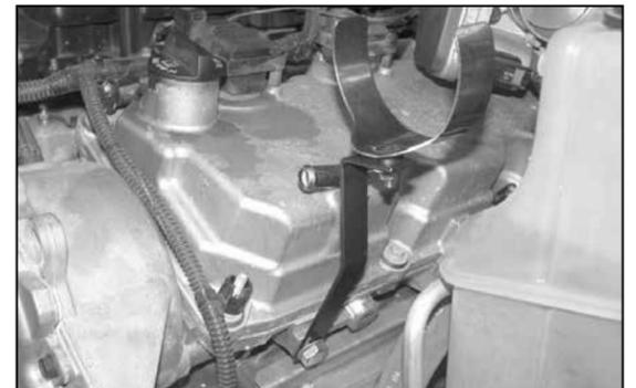
8. Using the provided hardware, install the tube-mounting bracket onto the engine at the threaded hole in the cylinder head as shown.
