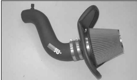
18. Install the air filter assembly onto the K&N® intake tube as shown.
