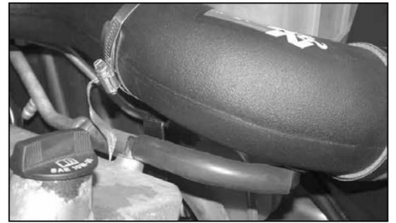
21. Install the provided silicone vent hose onto the valve cover vent and onto the elbow into the K&N® intake tube as shown.
