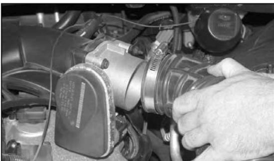
3. Loosen the hose clamp that secures the intake tube to the throttle body and pull the intake tube off the throttle body.
