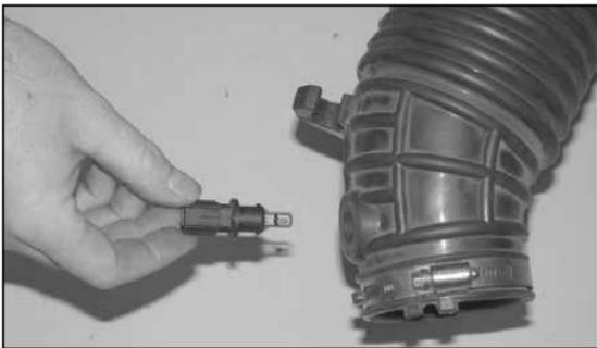
13. Remove the air temperature sensor from the factory intake tube.
