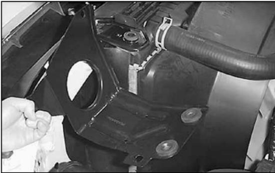
10. Remove the air cleaner mounting bracket.
