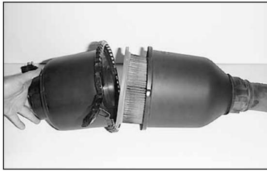
14. Disassemble the air cleaner assembly.
