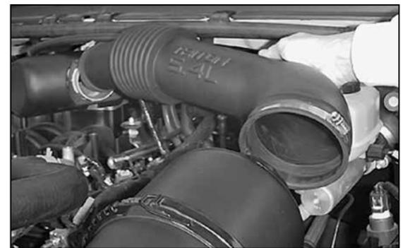
7. Remove the stock intake tube.
