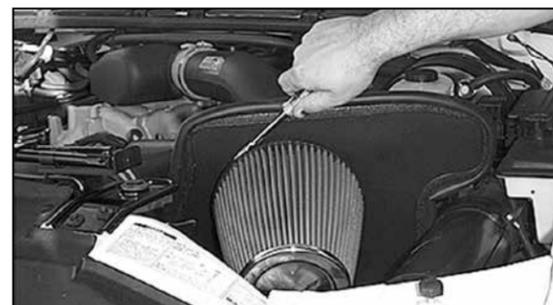
37. Install the air filter and tighten hose clamp.
