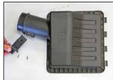
10. Remove the two screws securing the mass air sensor, then remove the mass air sensor from the upper air box housing as shown.
