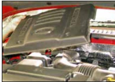
4. Remove the engine cover as shown.
