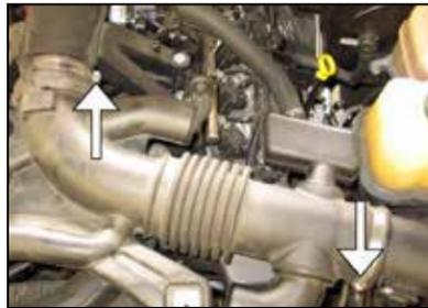
5. On the factory inlet tube, loosen the hose clamps at the upper air box housing and at the throttle body inlet.
