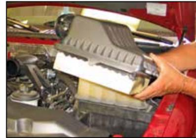
8. Remove the upper air box housing and air filter from the lower air box housing as shown.
