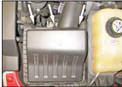
7. Un-snap the three latches securing the upper air box housing to the lower air box housing as shown.
