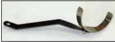
19. Install the saddle clamp onto the tube bracket (#06508) and secure with the provided hardware.
