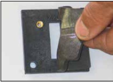
11. Install the provided gasket onto the mass air sensor adapter as shown with the sticky side down.
