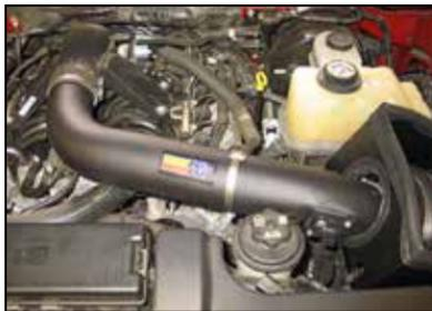
24. Install the intake tube into the air filter assembly and silicone hose at the engine inlet tube, then align with the tube bracket and secure with the provided hose clamps as shown.
