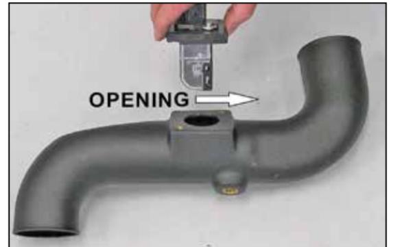
19. Install the mass air sensor assembly into the K&N intake tube and secure with the provided hardware.
