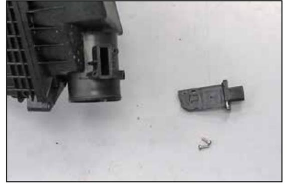
17. Remove the mass air sensor from the factory air box.
