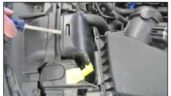
6. Using a flat blade screw driver, gently pry up the fresh air scoop to release it from the locking tab. Then push it towards the rear of the vehicle to release it from the Fresh air intake.
