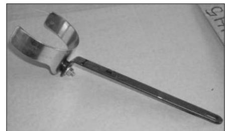
14. Vehicles that come equipped with manual transmissions assemble the large "L" bracket onto the saddle bracket as shown.
