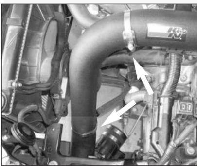
26. Line up the two saddle brackets onto the intake tube then secure the tube with the provided hose clamps.
