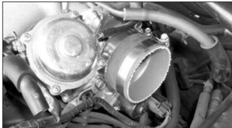
10. Install the silicone hose, (08756), onto the throttle body with the provided hose clamps as shown.
