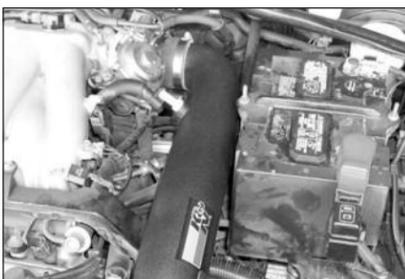
25. Install the new K&N intake tube onto the throttle body. Do not tighten hose clamps completely at this time.
