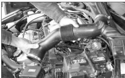
5. Remove the air intake tube as shown.
