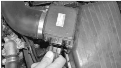
2. Disconnect the mass air electrical connection as shown.
