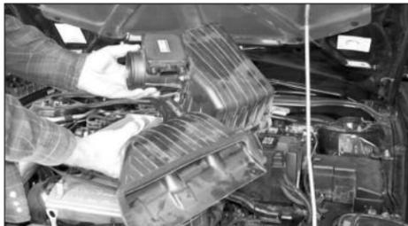
9. Remove the complete air box from vehicle as shown. **NOTE: K&N Engineering, Inc., recommends that customers do not discard factory air intake.**
