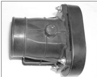
20. Install the K&N filter adaptor onto the mass air sensor with the hardware provided.
