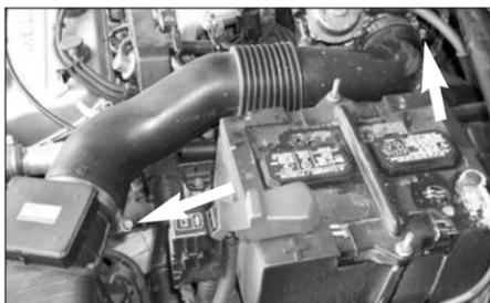
4. Loosen the hose clamp at the throttle body and air box assembly.
