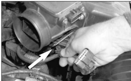
6. Remove electrical wires from air box as shown.
