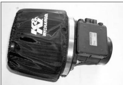
22. Install the provided dry charger onto the K&N filter as shown.
