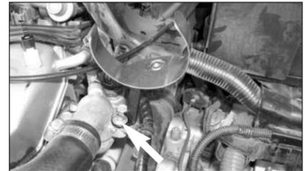
13. Secure the saddle bracket assembly onto the water neck with the provided bolt as shown.
