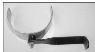
15. Vehicles that come equipped with automatic transmissions, assemble the saddle bracket as shown.
