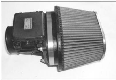
21. Install the new K&N filter charger onto the mass air sensor as shown.
