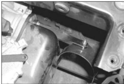
15b. Install saddle bracket assembly onto the transmission with the provided 10mm bolt.
