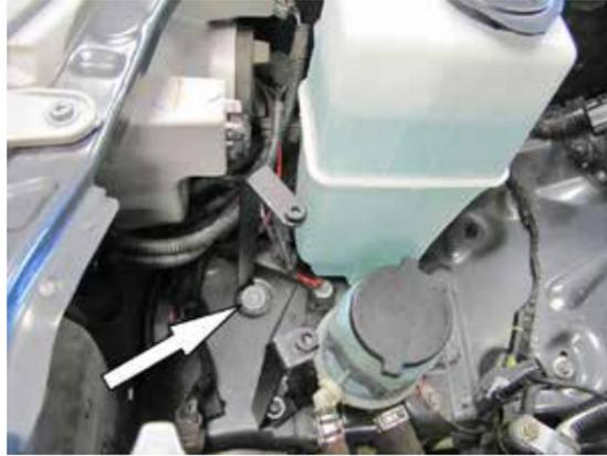
13. On vehicles equipped with secondary air injection, install the provided secondary air pump mounting bracket (083169) onto the inner fender using the provided hardware.
