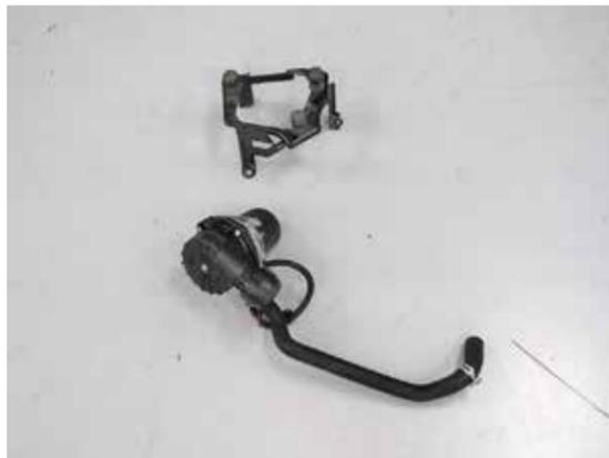
14. On vehicles equipped with secondary air injection, separate the secondary air pump mounting bracket from the pump motor.
