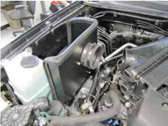
25. Install the provided coupling hose (08761) onto the filter adapter and secure with the provided hose clamp.
