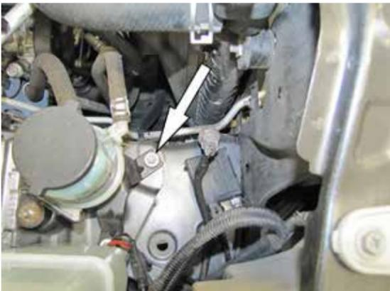
11. On vehicles equipped with secondary air injection, remove the power steering reservoir mounting bolt shown.
