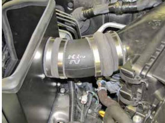
27. Install the K&N® intake tube into the hose at the filter adapter, align the hump hose with the air filter lid and then slide the hump hose onto the lid. Adjust the tube for proper fit and then secure with the provided hose clamps.
