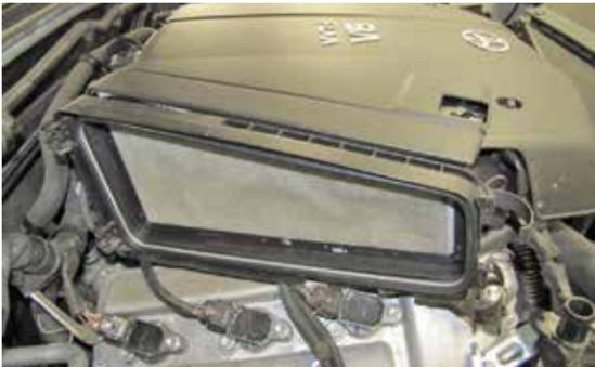
9. Install the gasket assembly into the air box.
