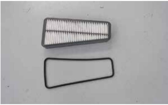
7. Remove the gasket from the factory air filter.
