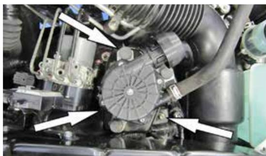
3. On vehicles equipped with a secondary air pump, remove the three bolts securing the bolts securing the secondary air pump and then disconnect the electrical connection and remove the secondary air pump from the engine compartment.
