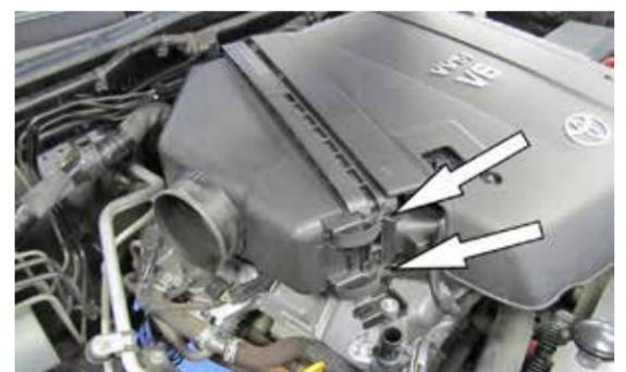
6. Release the two air box lid mounting clips and then remove the air box lid and factory air filter.
