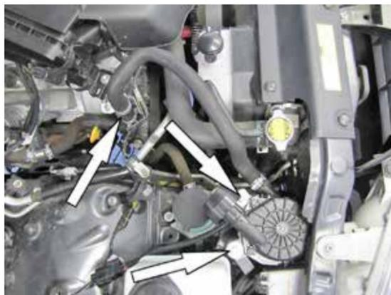
15. On vehicles equipped with secondary air injection, install the secondary air pump onto the brackets previously installed and secure with the provided hardware. Reconnect the secondary air hose to the fitting and secure with the factory spring clamp.
