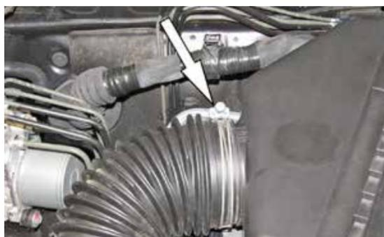
4. Loosen the hose clamp securing the intake hose to the air filter housing.
