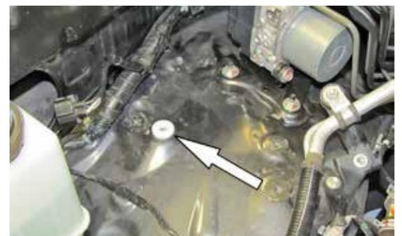
21. On 2012 and later model year vehicles, set the provided nylon spacer onto the inner fender heat shield mounting location as shown.
