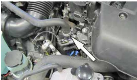
2. On Vehicles equipped with a secondary air pump, release the spring clamp securing the secondary air hose to the union on the engine and then disconnect the secondary air hose.
