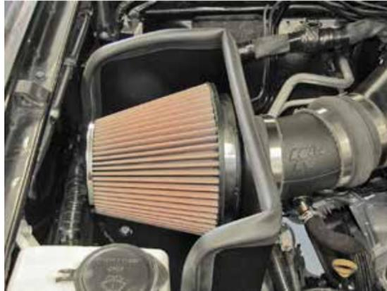
28. Install the K&N® air filter onto the filter adapter and secure with the provided hose clamp.
