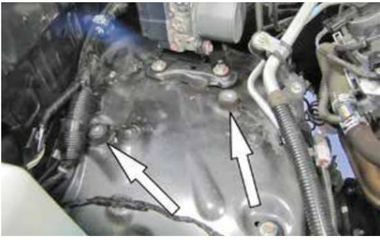
22. On 2005 through 2011 model year vehicles, install the two 6mm rubber mounted studs onto the inner fender as shown.
