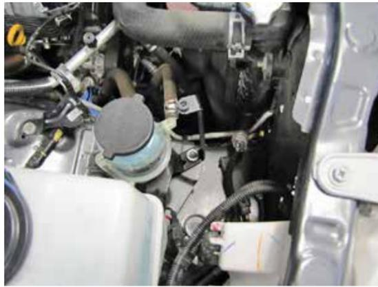
12. On vehicles equipped with secondary air injection, install the provided secondary air pump mounting bracket (083168) onto the power steering reservoir mount and secure with the factory retaining bolt from the previous step.
