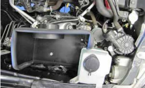
23. Set the heat shield onto the inner fender and secure with the provided hardware.
