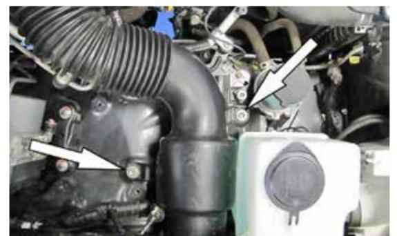
5. Remove the two bolts securing the resonator chamber to the inner fender and then remove the chamber and hose from the vehicle.
