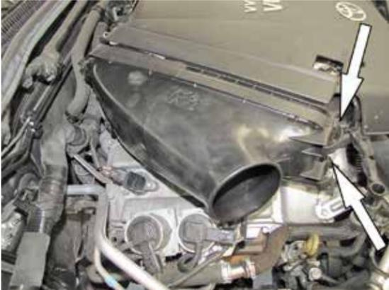
10. Install the K&N® air filter lid onto the air box and secure with the factory retaining clips.
