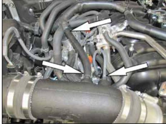
11. Install the crank case vent hose assembly into the factory crank case vent hose and then connect the open end to the fitting installed into the K&N® intake tube. Connect the factory fuel pressure regulator vent hose into the fitting installed into the K&N® intake tube.
