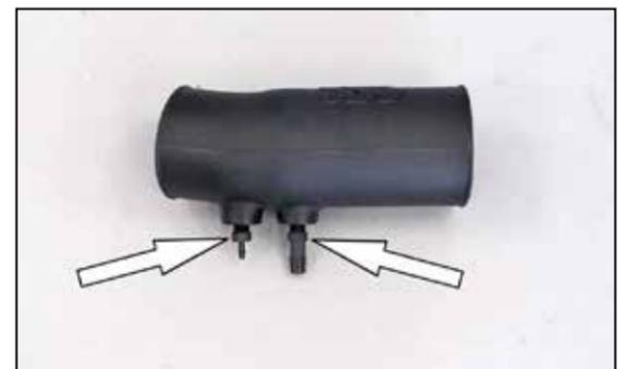
6. Install the two provided vent fittings into the K&N® intake tube as shown.
