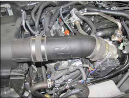
9. Install the K&N® intake tube assembly into the coupling hoses, secure the air box lid with the factory retaining clips and then secure the tube with the provided hose clamps.
