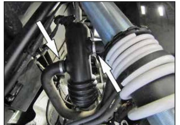
6. Release the clamps that secure the BOV hose and crank case vent hose to the intake tube and then disconnect the hoses from the tube.
