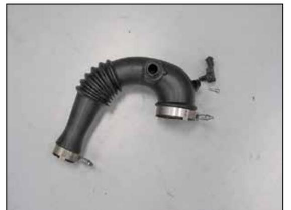
20. Remove the inlet temperature sensor from the factory intake tube.
