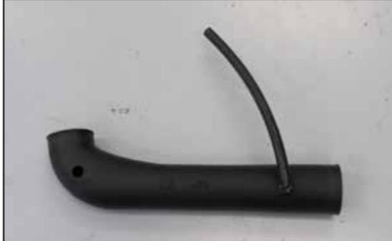
26. Install the provided crank case vent hose onto the fitting as shown.
