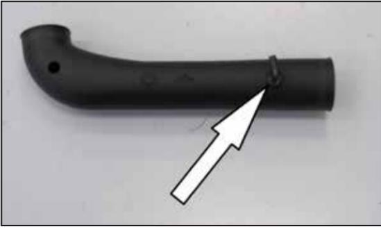
25. Install the 90°, 1/2" vent fitting into the K&N® intake tube as shown.
