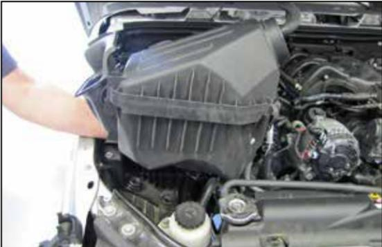
8. Lift up and remove the air filter housing from the vehicle.
