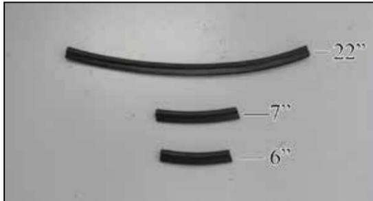
14. Cut the provided edge trim into three sections. One section is to be 6" long, one section is to be 7" long and the final section is to be 22" long.
