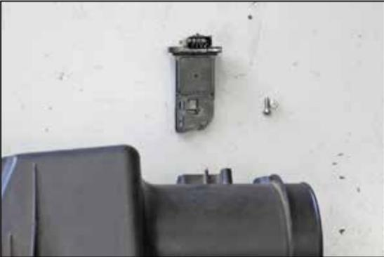
27. Remove the two screws securing the mass air sensor into the factory air box and then remove the sensor from the air box.
