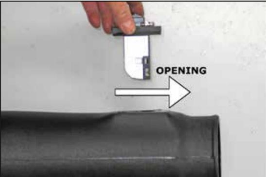
29. Install the mass air sensor assembly into the K&N® intake tube as shown and secure with the provided hardware.
