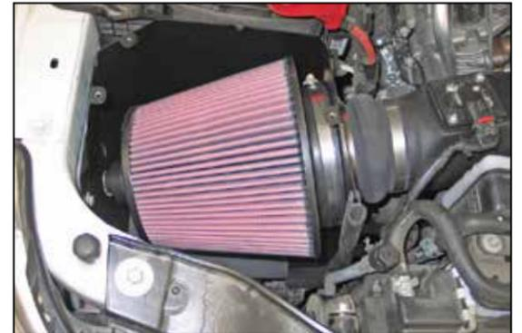
38. Feed the K&N® air filter top first into its location, then rotate it back and install onto the filter adapter. Secure the air filter with the provided hose clamp.
