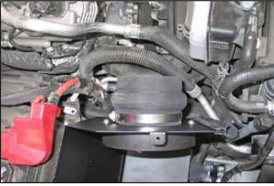
25. Install the silicone hump hose (08418) onto the filter adapter and secure with the provided hose clamp.
