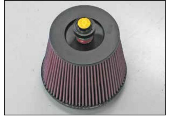
37. Install the filter minder along with the provided grommet into the K&N® air filter as shown.
