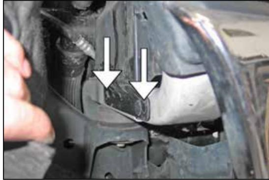
16. Remove the two clips shown that retain the bottom of the fresh air intake duct.
