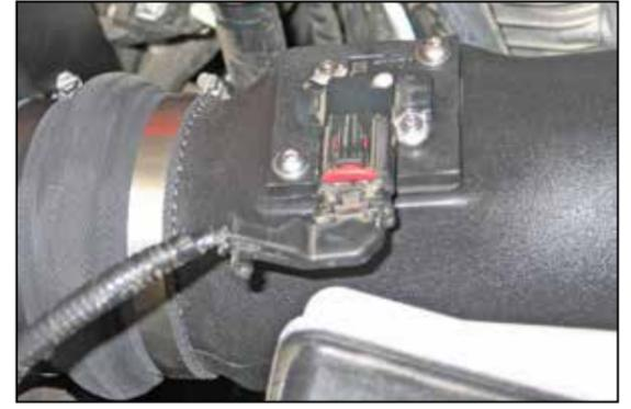
35. Reconnect the mass air sensor electrical connection. Secure the mass air sensor wiring harness to the A/C recharge pipe with the provided tie wrap.
