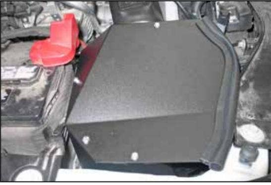
40. Attach the heat shield lid onto the heat shield and secure with the provided hardware.
