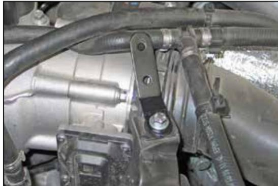
33. Install the coolant hose bracket onto the fan shroud as shown using the provided hardware.
