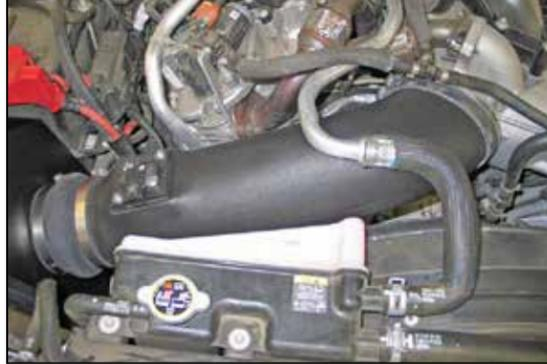
31. Install the intake tube into the silicone hose attached to the filter adapter and align the tube with the factory intake. Slide the silicone hose onto the factory intake and then secure the tube with the hose clamps.
