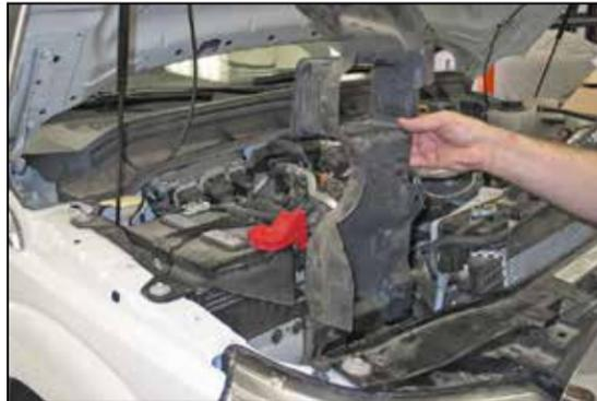
19. Remove the fresh air intake duct from the vehicle. Secure the inner fender to the vehicle with the original hardware from step #15.
