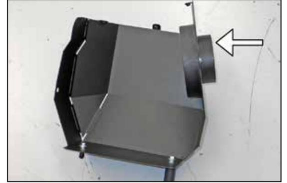
21. Install the filter adapter into the heat shield using the provided hardware.
