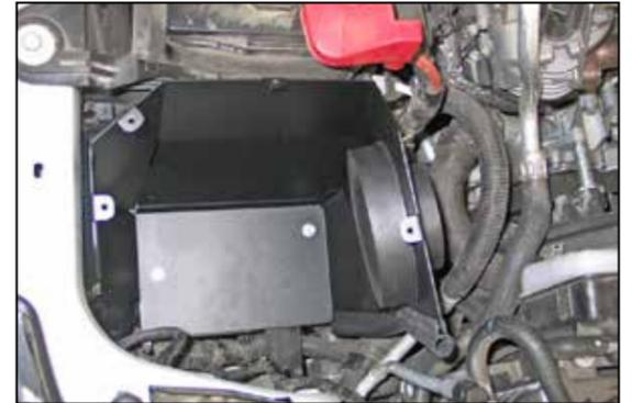
24. Set the heat shield assembly into position and secure with the factory mounting hardware from step #12.
