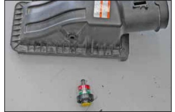
36. Remove the filter minder from the factory upper air box.
