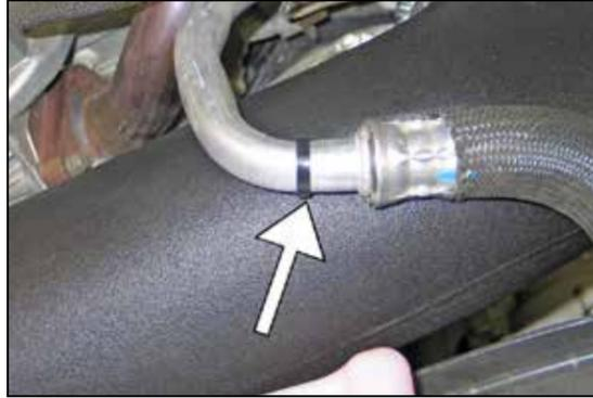
32. Secure the coolant pipe to the insert of the K&N® intake tube with the provided mounting tie wrap.
