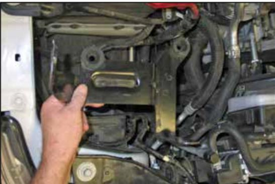
13. Remove the air box mounting bracket from the vehicle.
