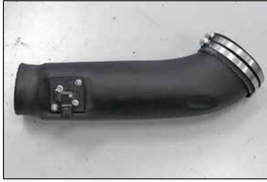
30. Install the provided silicone hose (08540) all the way onto the K&N® intake tube so the end of the tube is exposed.
