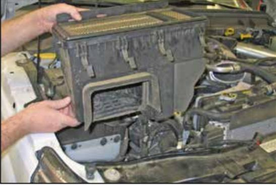
11. Remove the lower air box from the vehicle.
