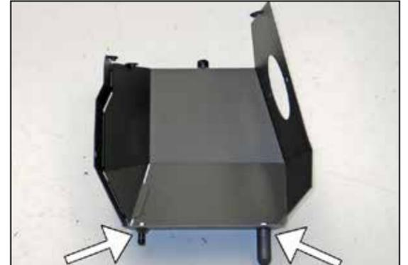
20. Install the two heat shield stand-offs onto the heat shield as shown using the provided hardware.
