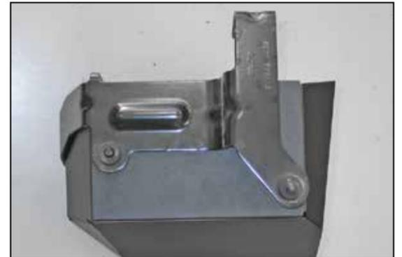
22. Install the factory air box mounting bracket onto the heat shield as shown so that the mount stand-offs installed in step #20 snap into the factory mounting grommets.
