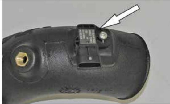
14. Remove the sealing O-Ring from the sensor and then install the sensor into the K&N® intake tube and secure with the provided hardware.
