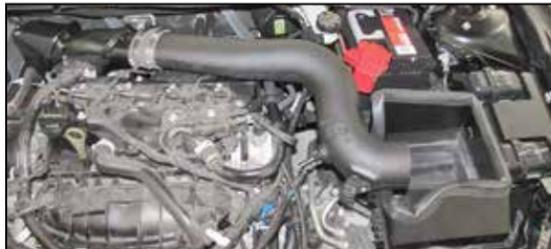
16. Install the K&N® intake tube into the coupling hose at the turbo inlet and align with the tube mounting bracket installed in step #8. Secure the tube with the provided hose clamp and hardware.
