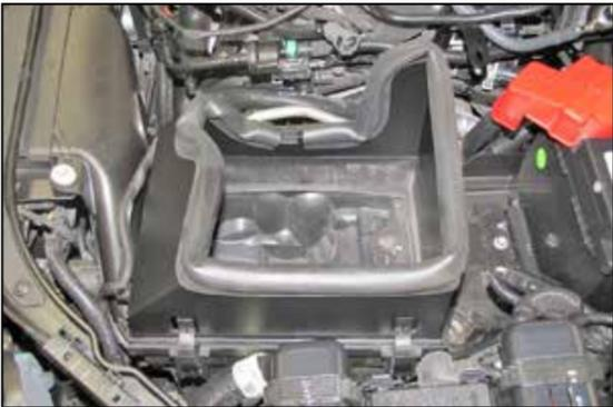
11. Install the heat shield assembly onto the lower air box and secure with the factory retaining clips.
