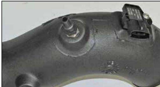
15. Install the quick disconnect fitting into the K&N® intake tube as shown.
