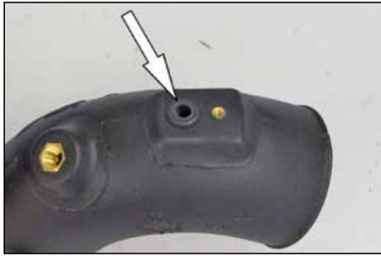
13. Install the provided grommet into the K&N® intake tube as shown.
