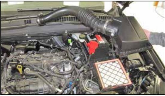
7. Lift up and remove the upper air box housing and intake tube from the vehicle. Remove the stock air filter.
