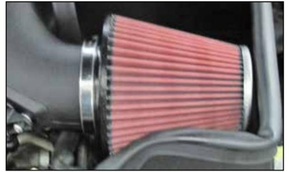
19. Install the K&N® air filter and secure with the provided hose clamp.
