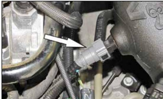
17. Connect the EVAP vent line to the quick disconnect fitting installed into the K&N® intake tube.
