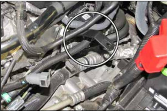
9. Be sure engine is completely cool before proceeding with this step. Remove the nut securing the thermostat housing (directly above the engine temperature sensor). Then install the provided tube mounting bracket and secure with the factory nut.
