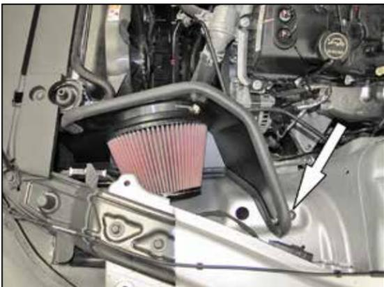
10. Flex the heat shield back and install the K&N® air filter onto the adapter then secure the filter with the hose clamp. Secure the upper heat shield mounting bracket with the hardware provided.
