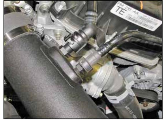
15. Connect the crank case vent and EVAP vent lines to the fittings installed into the K&N® intake tube.
