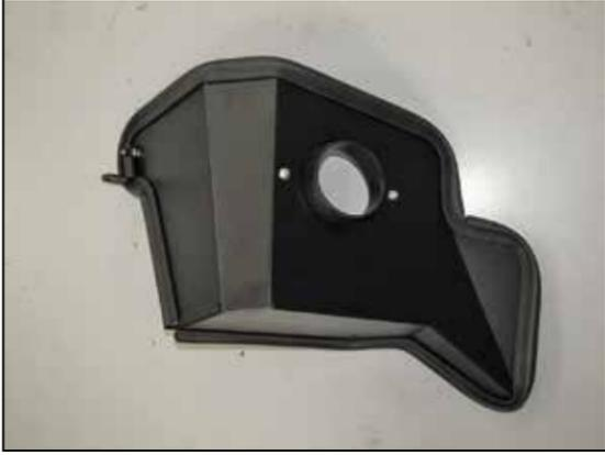
8. Install the provided mounting bracket (064326) and spacer onto the heat shield using the provided hardware.
