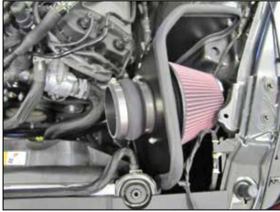
11. Install the provided hump coupler (08699) onto the filter adapter and secure with the provided hose clamp.
