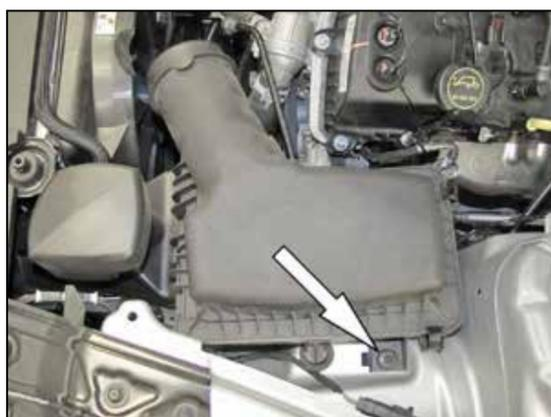
4. Remove the bolt securing the factory air filter housing and then remove the complete air filter housing from the vehicle.
