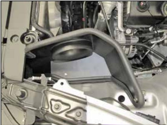
9. Install the heat shield onto the lower mounting bracket and then secure it only to the lower mounting bracket at this time.
