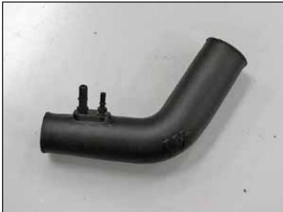
13. Install Quick disconnect fittings into the K&N® intake tube as shown.
