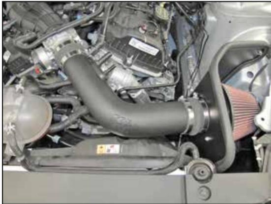
14. Install the intake tube fully into the hump coupler and then into the straight coupler at the throttle body, adjust the tube for best fit and then secure with the provide hose clamps.
