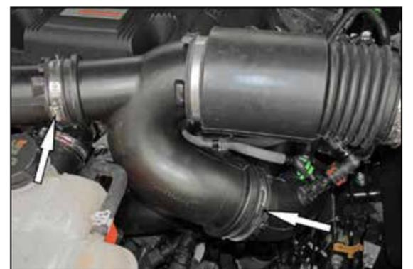
5. Loosen the two hose clamps that secure the factory intake tube to the turbo inlets, then remove the factory intake tube from the vehicle.
