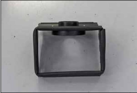
9. Install the K&N® filter adapter into the heat shield and secure with the provided hardware.
