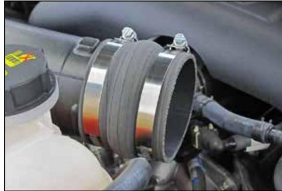
14. Install the provided coupler hose (087121) onto the passenger side turbo inlet hose and secure with the provided hose clamp.
