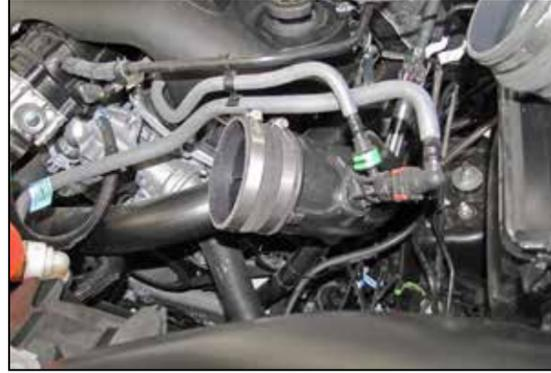
13. Install the provided coupler (08761) onto the driver's side turbo inlet tube and secure with the provided hose clamp.
