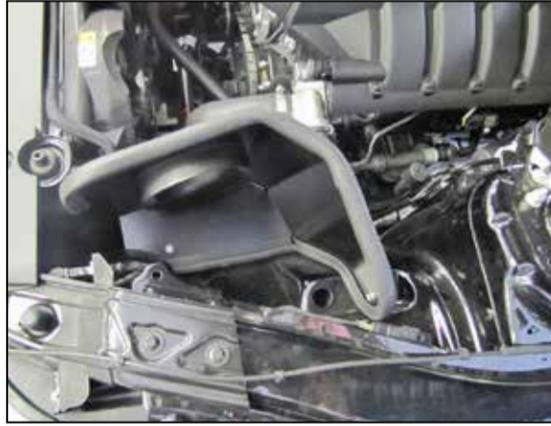
13. Install the heat shield assembly onto the inner fender and bracket and then secure with the provided hardware.
