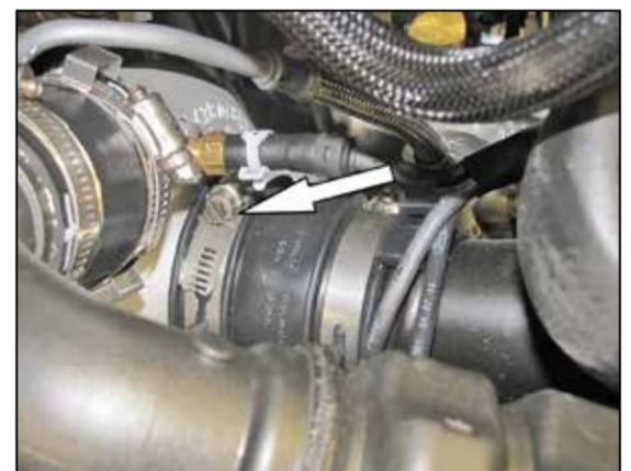
5. Loosen the hose clamp securing the intake tube to the Turbo.
