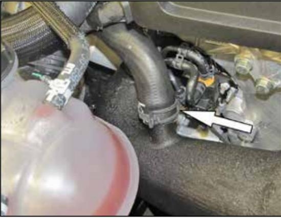
22. Install the BOV hose onto the K&N® intake tube and release the factory spring clip.
