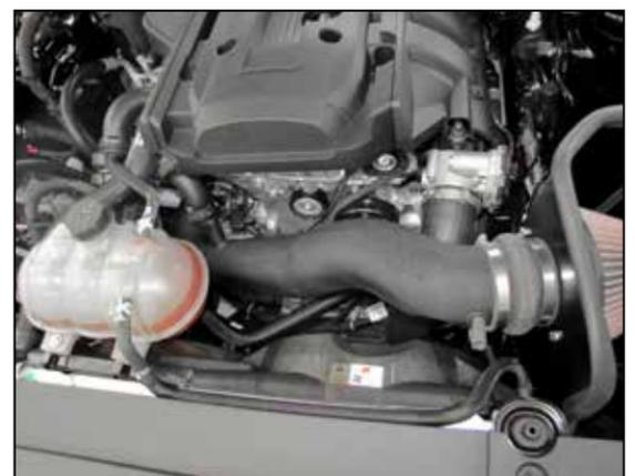
20. Slide the provided hump hose (08418) onto the end of the K&N® intake tube, then install the intake tube into the hose at the turbo inlet. Slide the hump hose into position on the filter adapter and secure the tube with the provided hose clamps.
