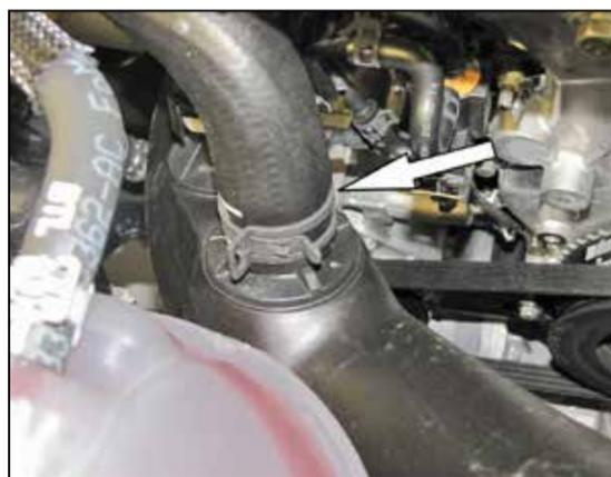
3. Using pliers, squeeze the spring clamp until it locks in the open position. Then disconnect the BOV hose from the intake tube.
