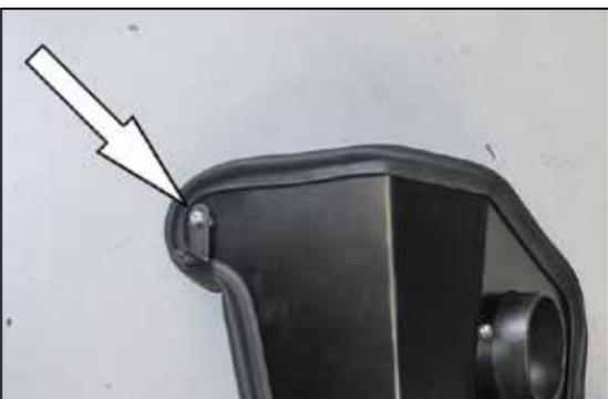
11. Install the heat shield mounting bracket (064326) onto the heat shield as shown.
