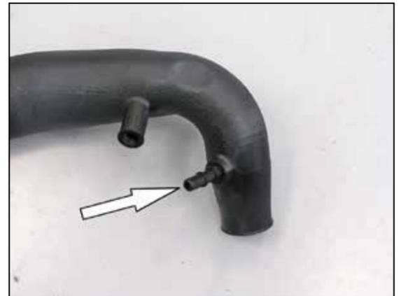
19. Install the provided quick disconnect fitting into the K&N® intake tube as shown.
