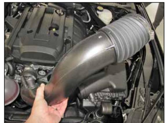
6. Remove the factory intake tube from the vehicle. **NOTE: K&N Engineering, Inc., recommends that customers do not discard factory air intake.**
