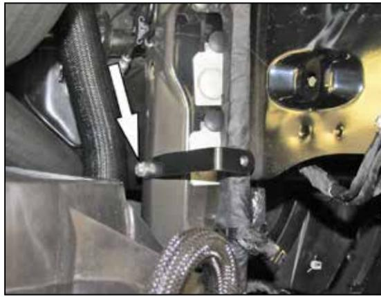
12. Install the heat shield mounting bracket onto the inner frame rail using the provided hardware.
