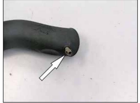
18. Remove the O-Ring from the factory temperature sensor and then install the sensor into the grommet installed into the K&N® intake tube.
