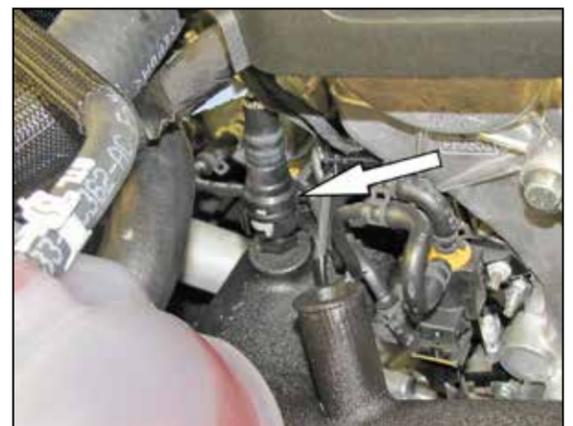
21. Connect the crank case vent hose to the fitting installed into the K&N® intake tube.
