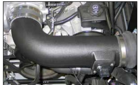
23. Install the K&N® intake tube assembly into the silicone hose at the filter adapter and then into the silicone hose at the throttle body and secure with the provided hose clamps.
