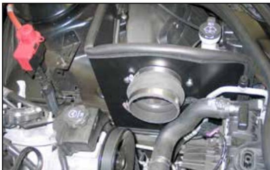
17. Install the silicone hose (08418) onto the filter adapter and secure with the provided hose clamp.
