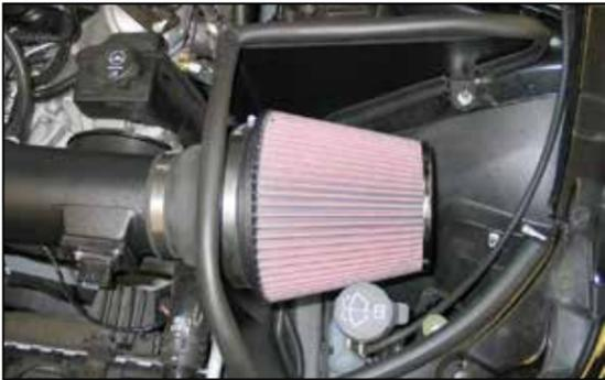
25. Install the K&N® air filter onto the filter adapter and secure with the provided hose clamp.
