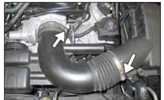
5. Loosen the hose clamps which secure the stock intake tube to the air box and throttle body.
