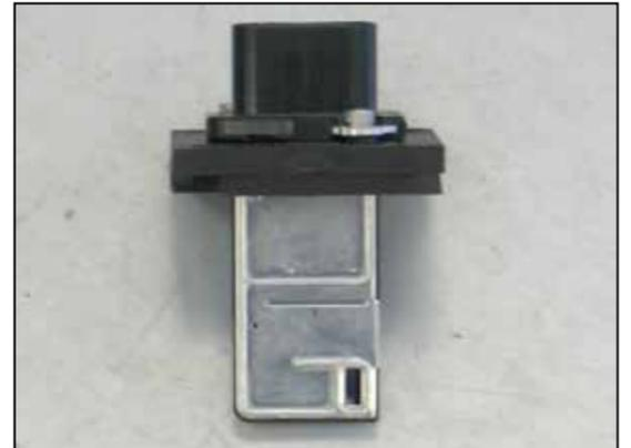
20. Install the mass air sensor into the adapter and secure with the provided hardware.
