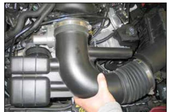
6. Remove the stock intake tube as shown.
