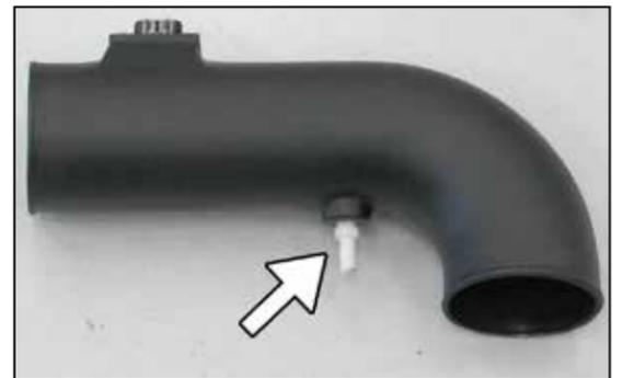
22. Install the provided 1/4 NPT fitting into the K&N® intake tube as shown.
