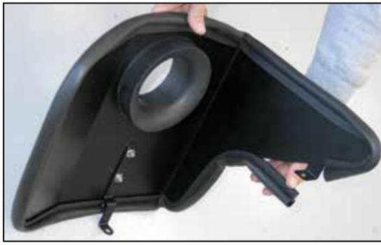
13. Install the edge trim onto the heat shield as shown.
