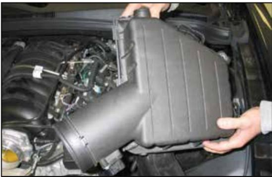
9. Lift up and remove the air box from the vehicle.
