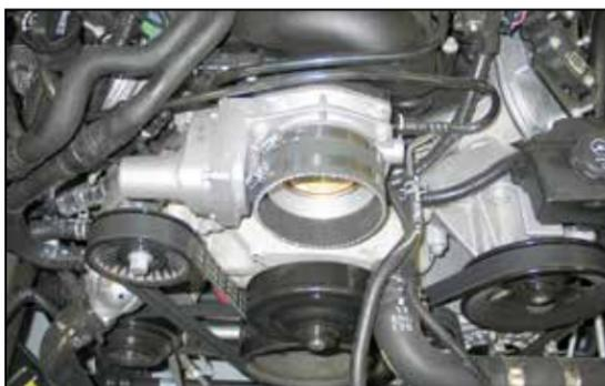
16. Install the silicone hose (08761) onto the throttle body and secure with the provided hose clamp.
