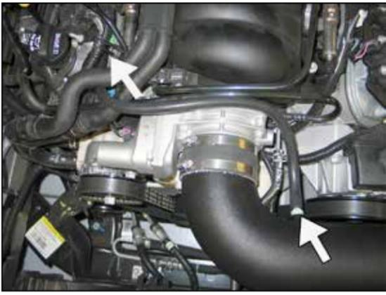
24. Attach the provided crank case vent hose to the 1/4" NPT fitting and then attach the open end to the vent port on the valve cover.
