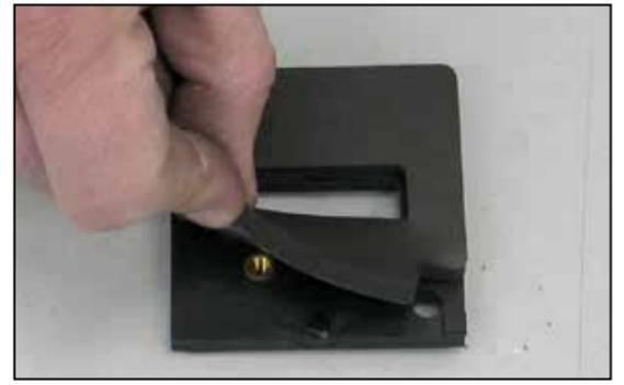
19. Install the provided gasket onto the mass air sensor adapter as shown.
