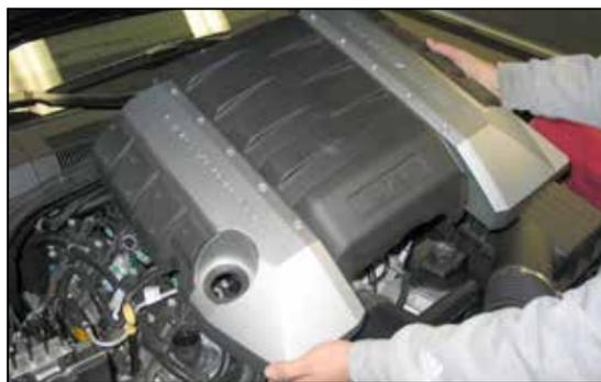
3. Remove the oil filler cap and then lift up and remove the engine cover. Reinstall the oil filler cap.
