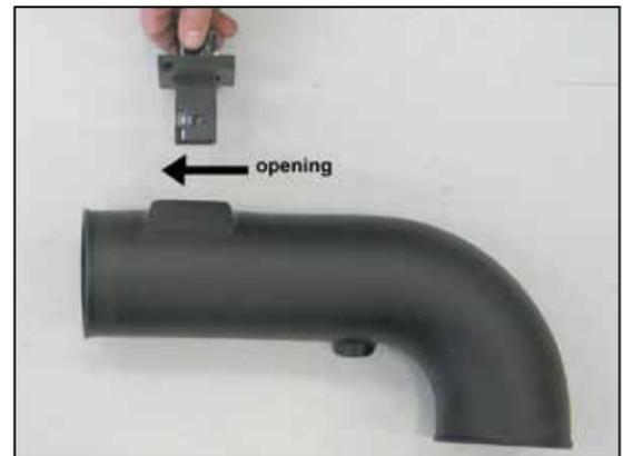
21. Install the mass air sensor assembly into the K&N® intake tube and secure with the provided hardware.
