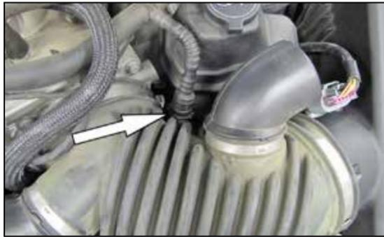
4. Release the locking tab and disconnect the crank case vent hose.
