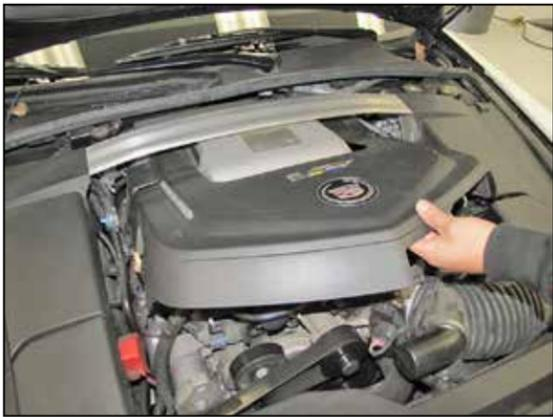
2. Lift up and remove the decorative engine cover from the engine.
