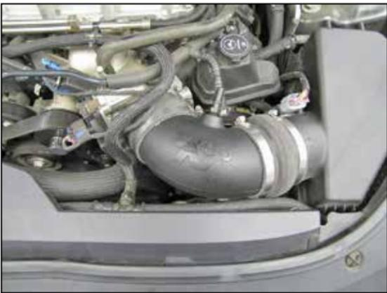
12. Install the K&N® intake tube into the hump coupler and then into the throttle body coupler. Adjust the tube for best fit and then secure with the provided hose clamps.
