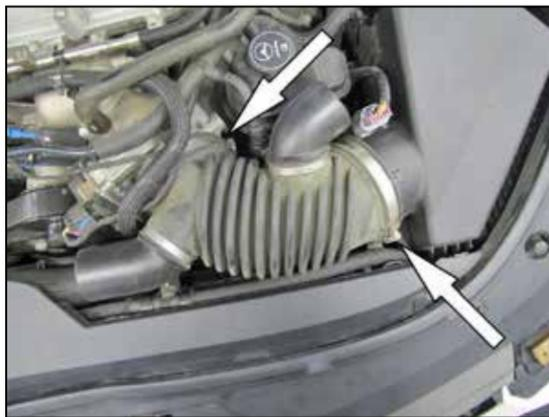
5. Loosen the two hose clamps securing the factory intake tube and then remove the intake tube from the vehicle.
