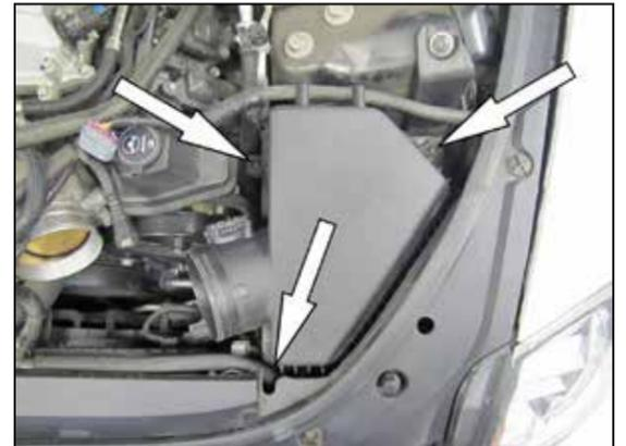
7. Loosen the three screws securing the upper air filter housing and then remove the housing and factory air filter.
