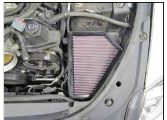
8. Install the provided K&N® air filter and re-secure the upper air filter housing with the factory screws. Reconnect the mass air sensor electrical connection.
