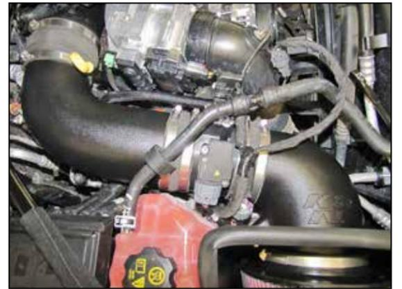
19. Connect the provided Mass air sensor extension harness into the factory harness and then reconnect the Mass air sensor and humidity sensor electrical connections.
