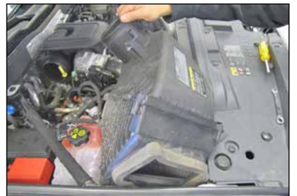
6. Lift up and remove the air box from the vehicle. **NOTE: K&N Engineering, Inc., recommends that customers do not discard factory air intake.**
