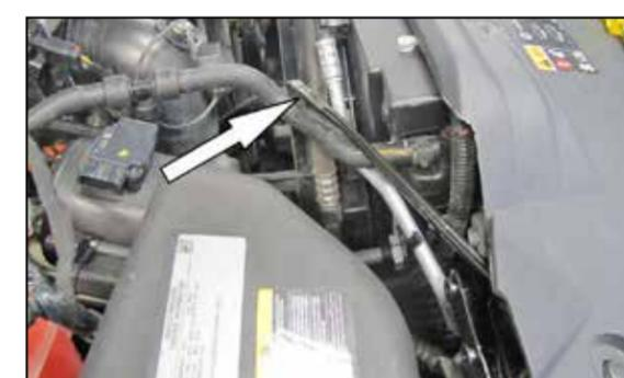
5. Loosen the bolt securing the fender brace to the core support then swing the brace clockwise towards the radiator for clearance.
