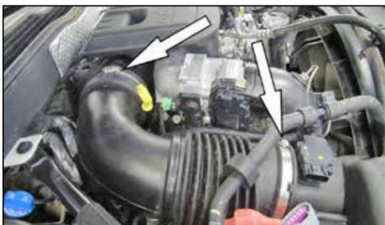
3. Loosen the hose clamps securing the factory intake hose to the air box and turbo inlet.
