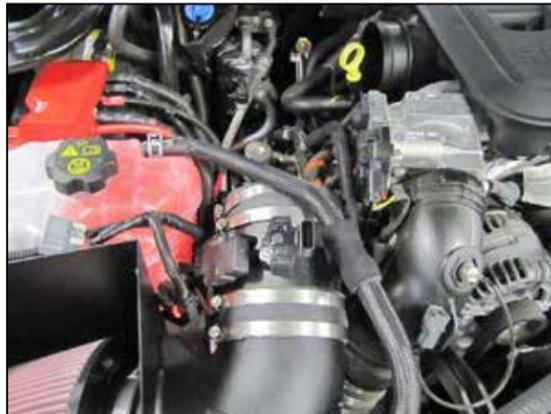
16. Install the Mass air assembly onto the K&N® intake tube as shown and secure with the provided hose clamps.
