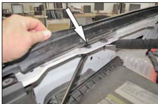
4. Lift up the hood seal trim and remove the bolt securing the fender brace.
