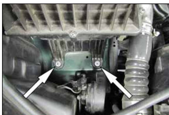
4. Remove the two nuts that secure the air filter housing to the inner fender.
