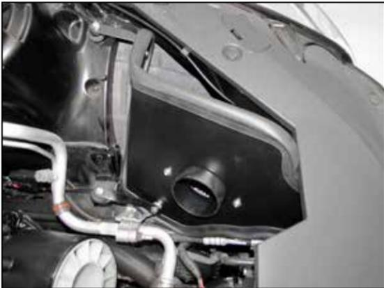
10. Install the heat shield assembly into the vehicle so that the mounting studs insert into the factory air box mounting grommets.
