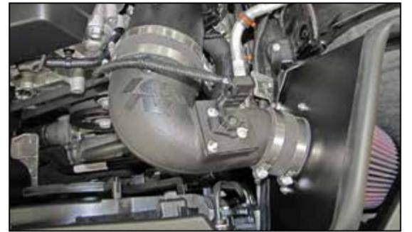
19. Reconnect the mass air sensor electrical connection and secure the wiring harness to the insert in the K&N® intake tube.
