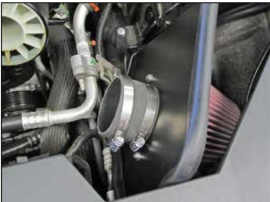
11. Install the provided coupler hose (08711) onto the filter adapter and secure with the provided hose clamp.
