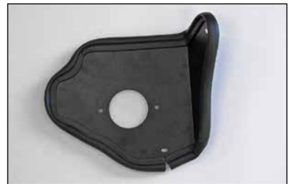
5. Install the provided edge trim onto the heat shield as shown.
