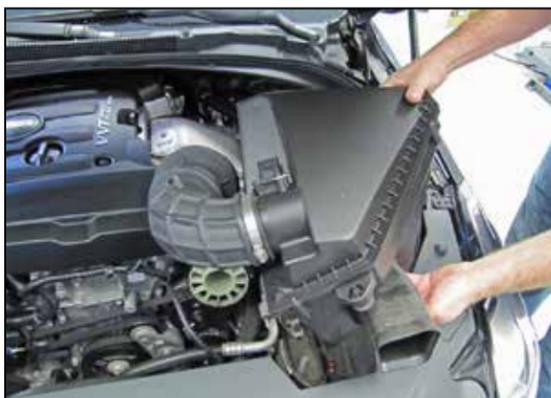
4. Lift the complete factory intake assembly up to dislodge it from the mounting grommets and then remove it from the vehicle.
