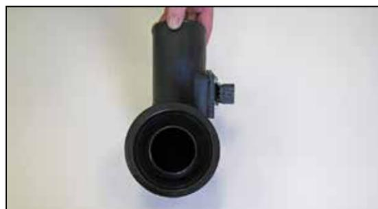
17. Install the air diverter into the K&N® intake tube so that the radius face is inside the intake tube.
