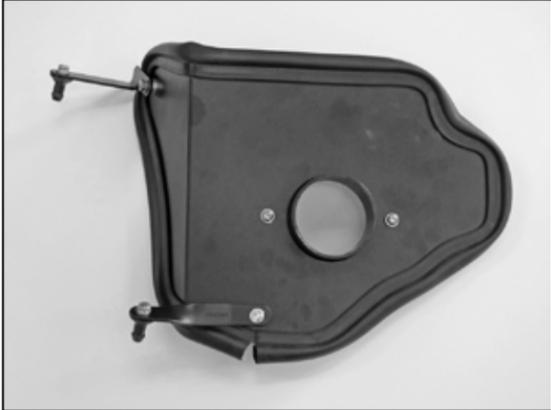
8. Install the mounting bracket assemblies onto the heat shield as shown and secure with the provided hardware.
