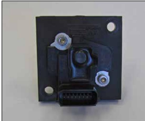
15. Install the mass air sensor into the K&N® mass air sensor adapter and secure with the provided hardware.
