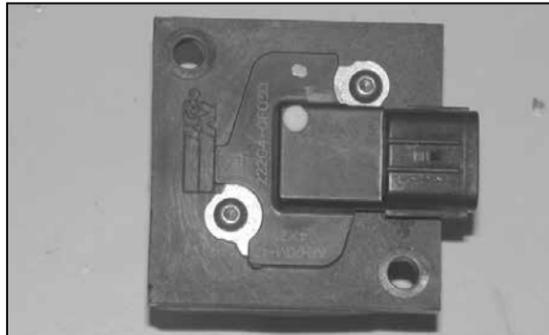
19. Install the mass air sensor into the K&N® mass air adapter and secure with the provided bolts as shown.
