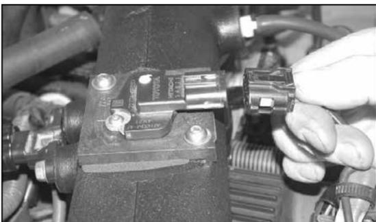
31. Reconnect the mass air sensor electrical connection as shown.
