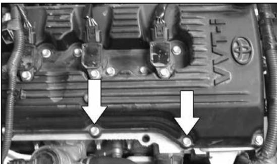
14. Remove the two valve cover bolts shown.
