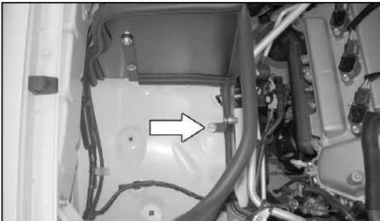
12. Install the heat shield onto the vehicle and secure with the provided hardware and nut removed in step #11.
