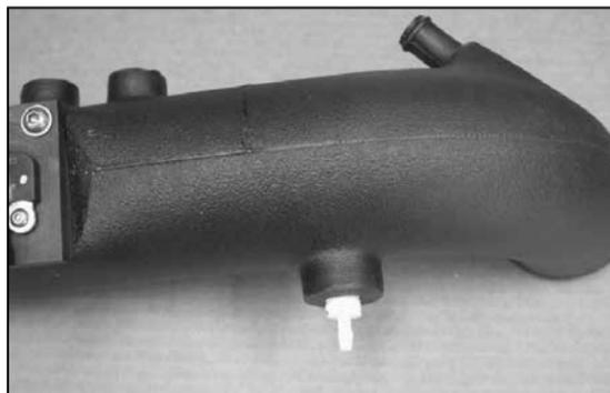
21. Install the supplied npt fitting into the K&N® intake tube as shown.
