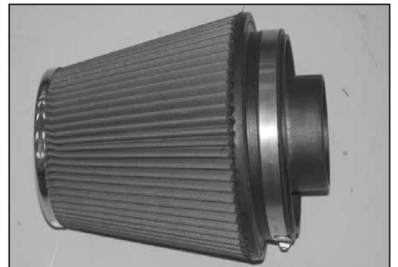
27. Install the radius filter adapter into the K&N® air filter and secure with the provided hardware as shown.
