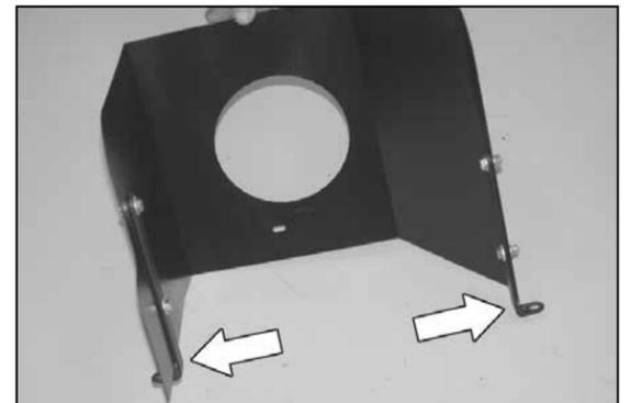
8. Install the two heat shield brackets (07159) onto the heat shield as shown with the provided hardware.
