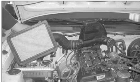
5. Unlatch the air box retaining clips, disconnect the fuel pressure regulator and crank case vent hoses, then lift the intake tract off of the throttle body as shown.
