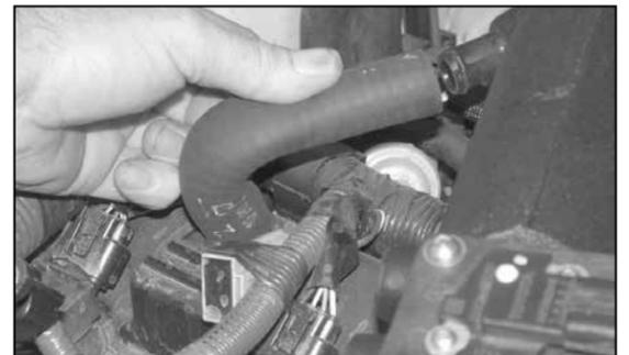
25. Install the provided crank case vent hose onto the valve cover port and then onto the K&N® intake tube as shown.
