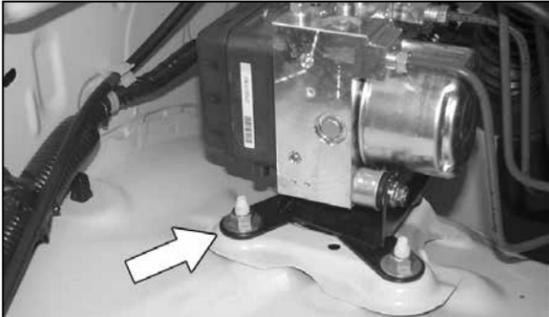
11. Remove the ABS pump mounting nut shown.
