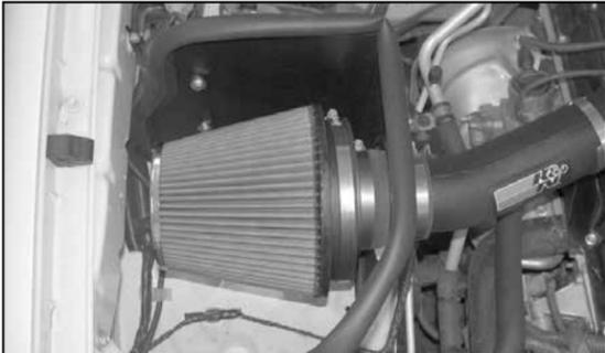
29. Install the K&N® air filter onto the intake tube as shown.
