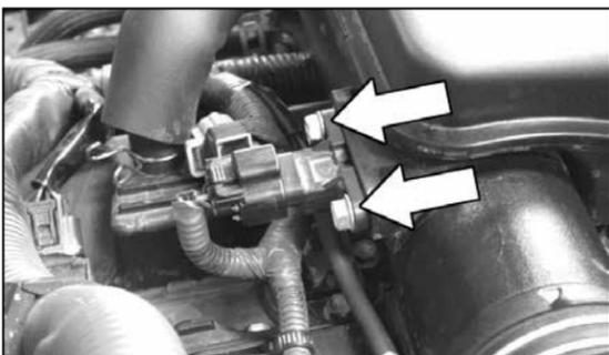
3. Remove the two bolts that secure the pressure sensor to the stock intake tube.
