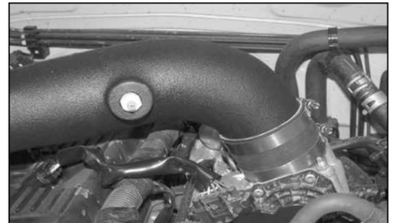
22. Install the K&N® intake tube onto the throttle body and align with the saddle bracket.
