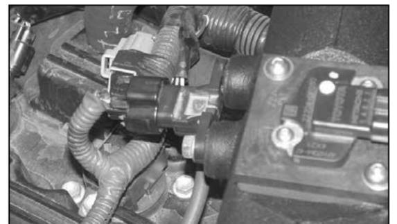
26. Install the pressure sensor onto the K&N® intake tube using the bolts removed in step #3.
