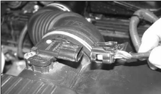
2. Disconnect the mass air sensor electrical connection and unclip the three wire harness retaining clips from the intake tract.
