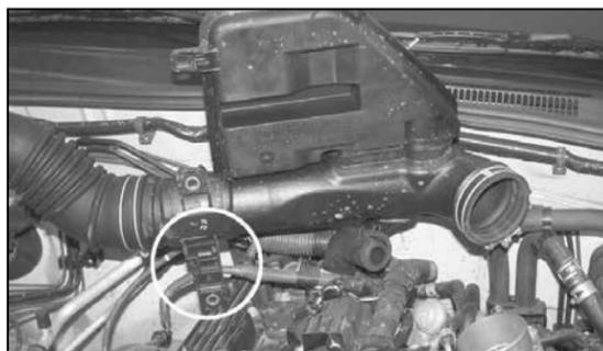
6. Disconnect the wire harness retaining bolts shown and then remove the lower air box from the vehicle.
