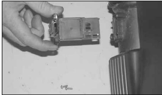
17. Remove the two mass air sensor retaining screws and then remove the mass air sensor from the factory air box.
