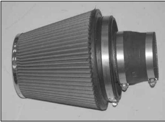
28. Install the provided silicone hose (08724) onto the K&N® air filter assembly and secure with the provided hose clamp as shown.
