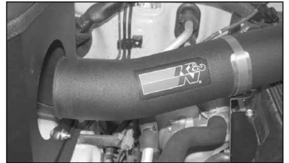
23. Secure the K&N® intake tube to the saddle bracket with the provided hose clamps. Also tighten the hose clamp securing the intake tube to the throttle body.
