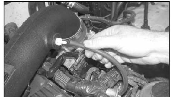
24. Install the provided vacuum hose onto the fuel pressure regulator and then onto the K&N® intake tube as shown.
