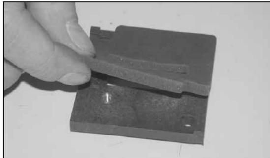
18. Install the supplied gasket onto the mass air sensor adapter as shown.
