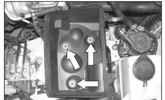
7. Remove the three-lower air box retaining bolts shown and then remove the lower air box from the vehicle.
