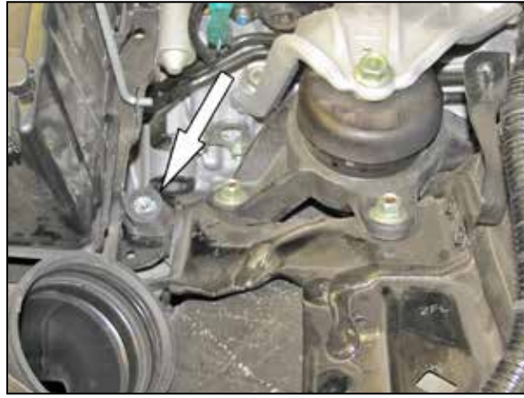
12. Install the provided rubber mounted stud onto the front air box mounting location as shown.
