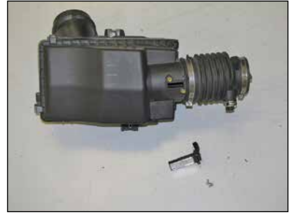
17. Remove the mass air sensor from the factory air box.
