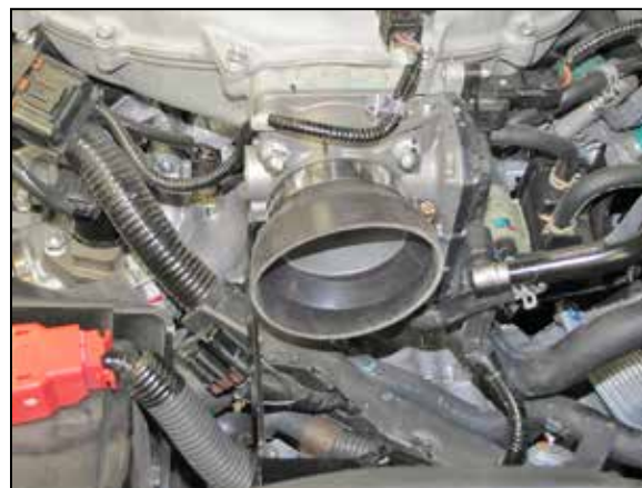
16. Install the appropriate step hose onto the throttle body and secure with the provided hose clamp. NOTE: The hose is a tight fit onto the throttle body.
