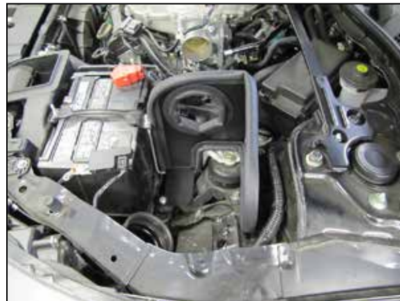
15. Set the heat shield into position on the rubber mounted stud and factory rear air box mounting location. Secure the heat shield with the provided hardware.
