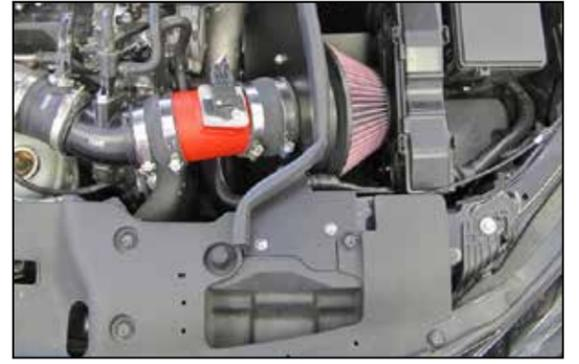
16. Install the provided fresh air duct and secure with the provided hardware. Install the remaining length of edge trim onto the fresh air duct.
