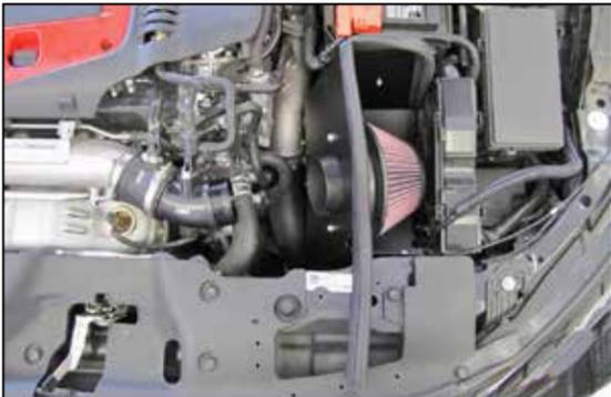
10. Set the heat shield assembly into position on the rubber mounted studs and then secure with the provided hardware.
