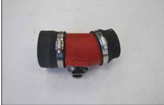
13. Install the provided coupler (084034) onto the outlet side of the K&N® intake tube and secure with the provided hose clamp.
