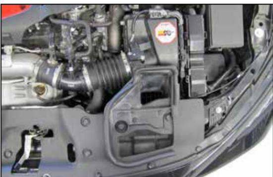
2. Disconnect the mass air sensor electrical connection and unhook the harness from the air filter housing.
