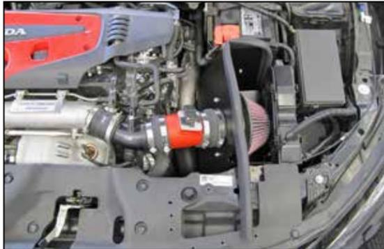
14. Install the intake tube assembly onto the turbo inlet and filter adapter, adjust the tube for best fit and secure with the provided hose clamp.
