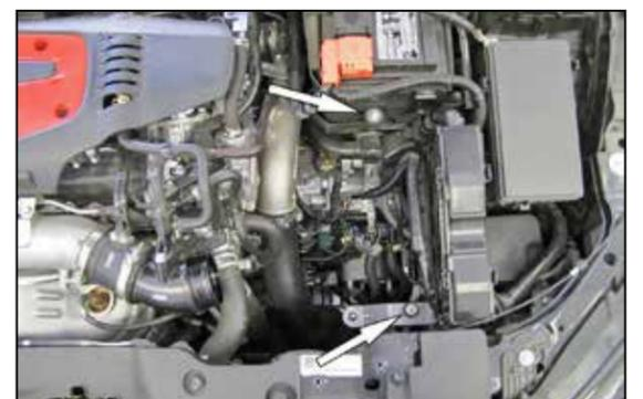
5. Install the two provided rubber mounted studs into the factory air filter housing mounting locations as shown.
