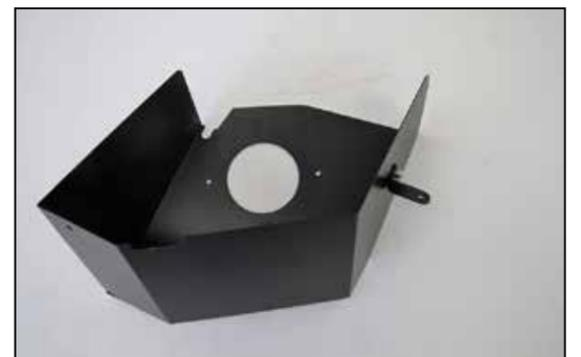
6. Install the provided mounting bracket onto the heat shield and secure with the provided hardware.
