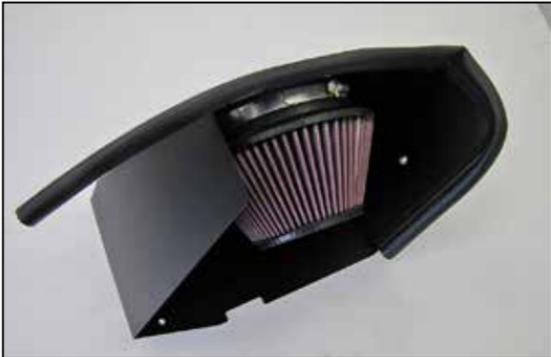
9. Install the K&N® air filter onto the filter adapter and secure with the provided hose clamp.
