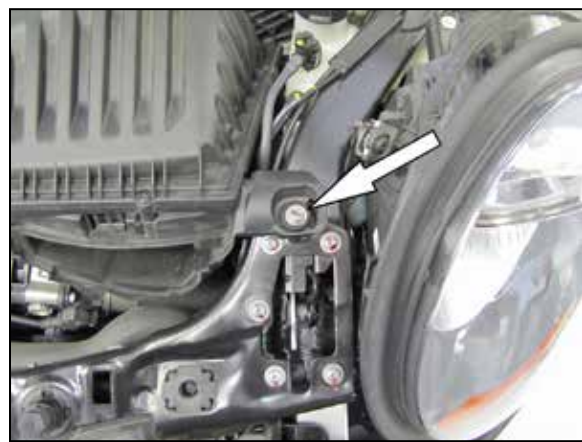
4. Remove the bolt shown that secures the air filter housing to the core support.
