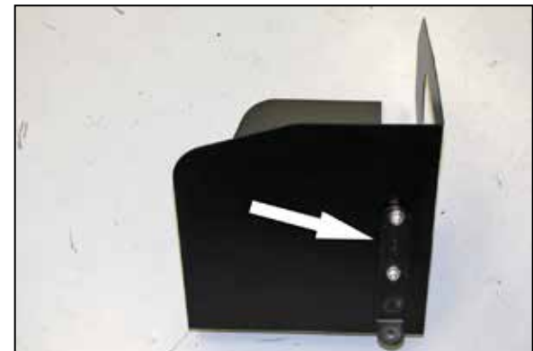
6. Install the heat shield mounting bracket (083172) onto the heat shield using the provided hardware.
