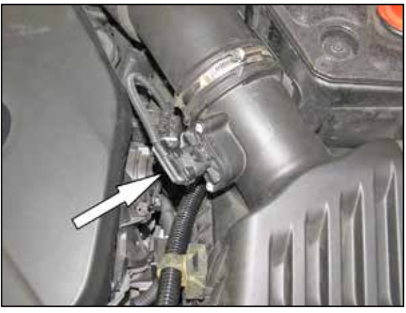
2. Disconnect the mass air sensor electrical connection.
