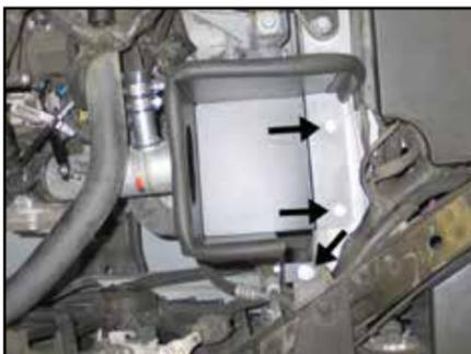
19. Install the heat shield assembly as shown. Secure the heat shield to the air box mounting locations with hardware provided.
