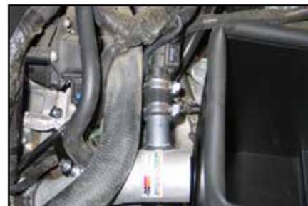
22. On vehicles equipped with an air injection pump, reroute the hose under the engine wiring harness and then connect it to the intake tube and secure with the provided hose clamp.
