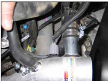
21. Reconnect the inlet air temperature sensor electrical connection.
