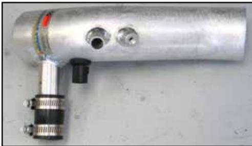
17. On vehicles equipped with an air injection pump, install the silicone hose onto the vent tube and secure with the provided hose clamp.
