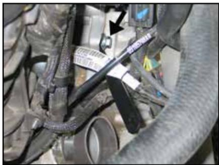
12. On 2010 model year and earlier vehicles, install the tube mounting bracket (06716) using the provided hardware.
