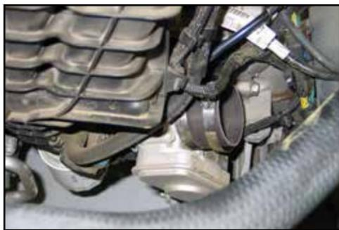
11. Install the provided silicone hose (08284) onto the throttle body and secure with the provided hose clamp.
