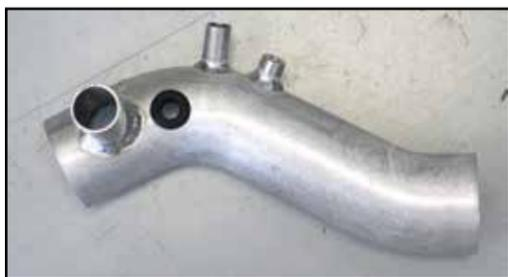
13. Install the provided temperature sensor grommet into the K&N® intake tube as shown.
