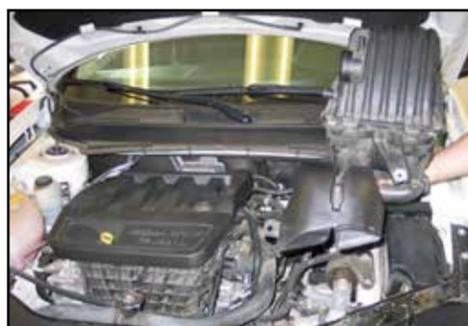
7. Lift up firmly on the air box to dislodge it from the mounting grommets and then remove the air box from the vehicle.
