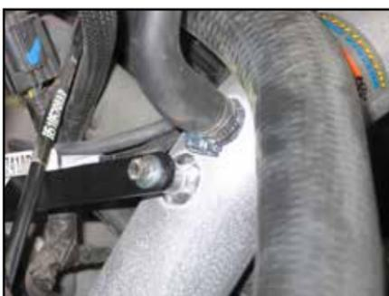
20. Attach the crank case vent hose to the K&N® intake tube and secure with the provided hose clamp.
