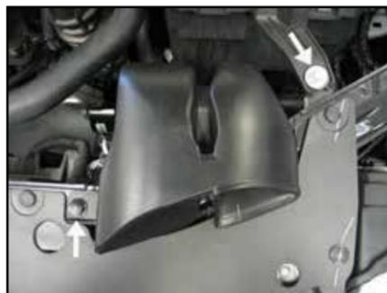
6. Remove the bolt which secures the air box to the radiator core support shown and then remove the plastic retaining clip which secures the fresh air inlet scoop.
