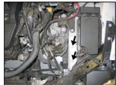
8. Remove the two air box mounting studs shown.
