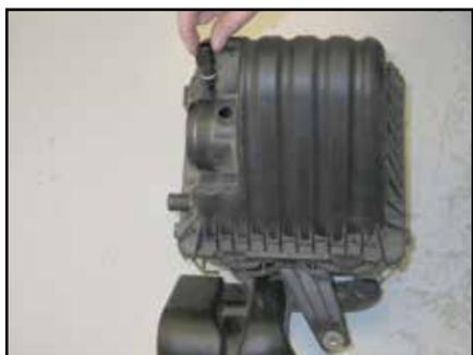
14. Remove inlet air temperature sensor from the stock air box and then remove the o-ring from the sensor.
