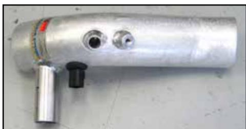
15. Install the air temperature into the grommet installed into the K&N® intake tube during step #13.
