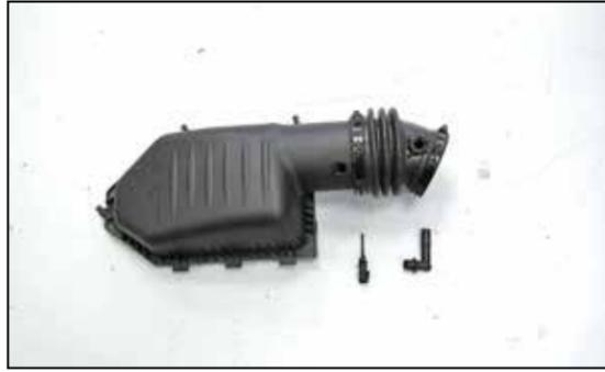
12. Remove the crank case vent and inlet air temperature sensor from the factory intake tube. **NOTE: The inlet air temperature sensor is very fragile, use care while removing the sensor.**
