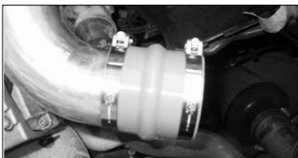
12. Install the hump hose approximately 2.5cm / 1" onto the intake tube and tighten the hose clip.
