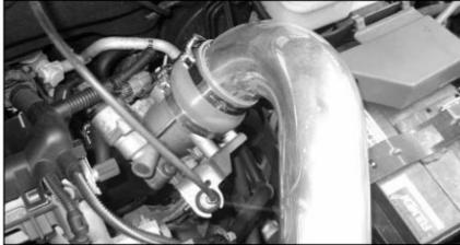
10. Install the longer two bend intake tube to the silicone stepped hose using a #300 barrel clamp supplied.
