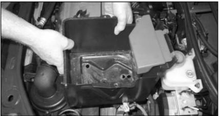
5. Carefully remove the battery tray from the vehicle.
