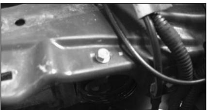
8. Fit the nut and washer to the top of the vibration mount.
