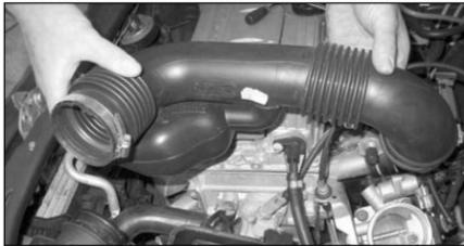
2. Undo the two hose clips and remove the intake tube from the vehicle.
