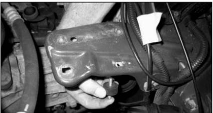
7. Fit the vibration mount to the stock air box mounting point.
