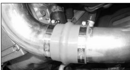
13. Install the second intake tube approximately 2.5cm / 1" into the hump hose.
