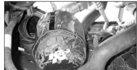
17. Fit the filter onto the end of the second intake tube using the hose clip supplied.
