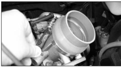
9. Fit the silicone stepped hose to the throttle body and tighten the #350 barrel clamp supplied.
