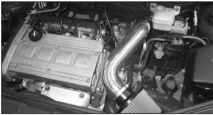
20. This K&N Typhoon intake kit has been designed to be used in two different configurations. In the case of inclement weather, the cold air tube can be removed and the filter can be clamped onto the first intake tube located in the engine compartment to avoid the possibility of ingesting water into the engine.
