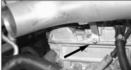
11. Install the bolt and washer through the bracket into the threaded hole in the valve cover and tighten the bolt, then tighten the hose clip on the stepped silicone hose.
