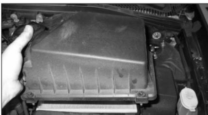
4. Remove the four bolts that secure the air cleaner cover, then remove the cover and filter as shown.
