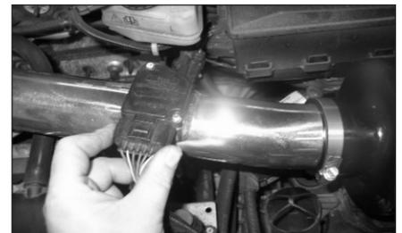
14. Reconnect the mass air sensor electrical connection as shown.
