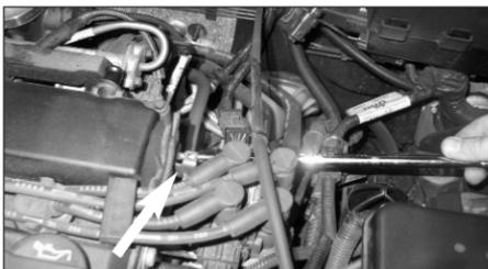
10. Remove the rear bolt on the ignition bracket as shown.
