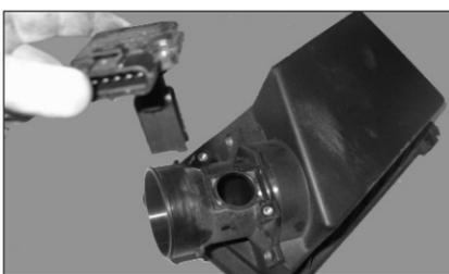
8. Remove the two bolts that secure the mass air sensor, then, remove the mass air sensor as shown.
