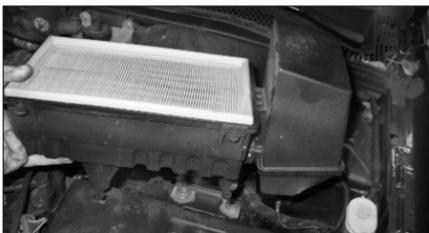
6. Pull firmly upwards to remove the lower air cleaner assembly as shown.
