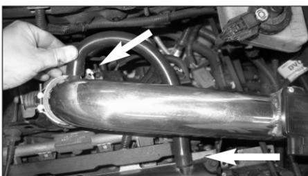
12. Using the provided vent hose, (Trim to fit), connect to the K&N Typhoon intake tube and valve cover as shown.
