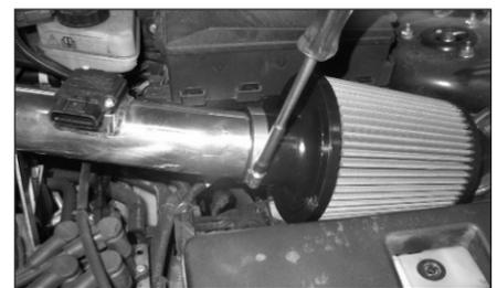
13. Install the K&N Filtercharger onto the K&N Typhoon intake tube and tighten with the provided hose clamp as shown.
