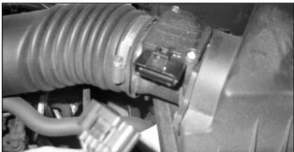
2. Disconnect the mass air sensor electrical connection as shown.
