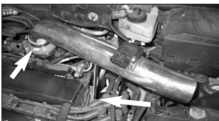
11. Install the K&N Typhoon intake tube into the silicone hose then line up the bracket with the ignition bracket and secure with the bolt from step 10 and tighten the hose clamps.
