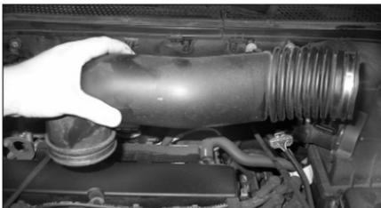
3. Loosen the hose clamps at the throttle body and at the mass air sensor, then, remove the stock intake tube as shown.
