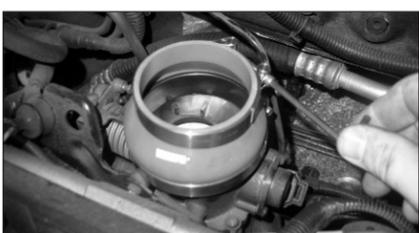
7. Install the provided silicone hose and hose clamps onto the throttle body as shown.
