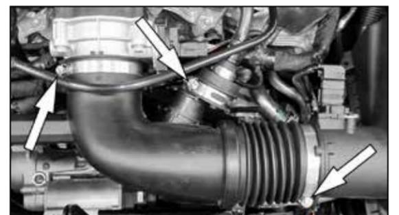
5. Loosen the three hose clamps that secure the intake tube and crank case vent tube then remove the tune from the vehicle
