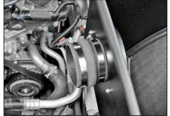
18. Install the provided hump coupler (084079) onto the filter adapter and secure with the provided hose clamp.
