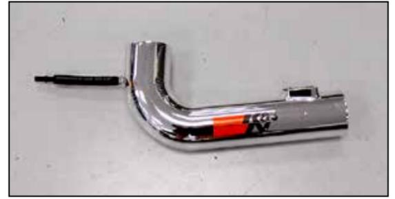
20. Install the EVAP hose assembly onto the K&N® intake tube as shown.
