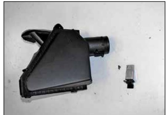
22. Remove the mass air sensor from the factory air filter housing.
