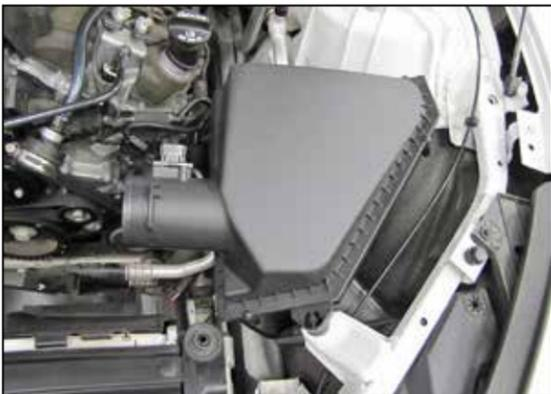
10. Lift up and remove the factory air filter housing assembly.
