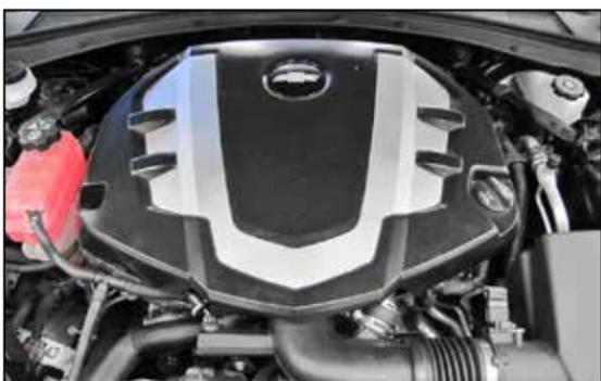
2. Remove the bolt that secures the decorative engine cover, remove the oil cap and then remove the decorative engine cover. Reinstall the oil cap.
