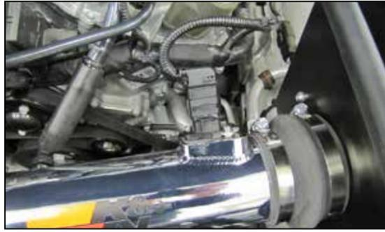
27. Reconnect the mass air sensor electrical connection.
