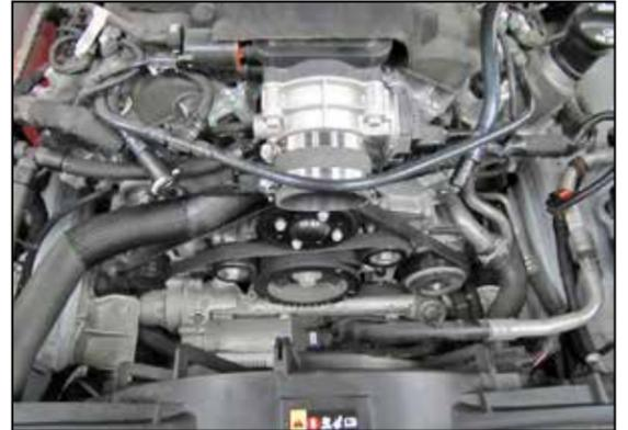
17. Install the provided coupler (084031) onto the throttle body and secure with the provided hose clamp.
