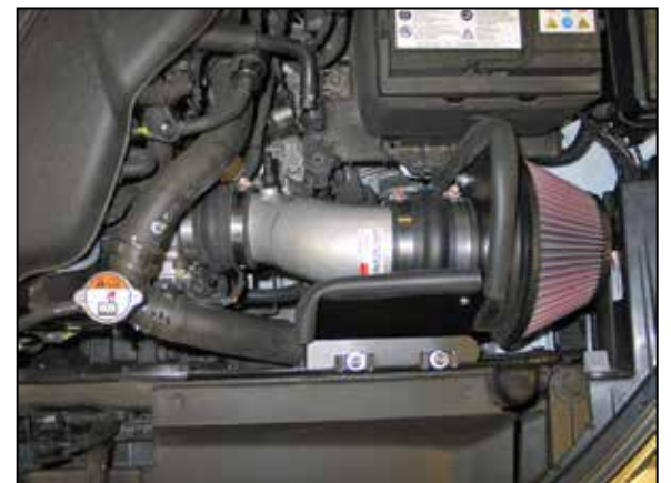
20. Install the K&N® intake tube into the silicone hose at the throttle body fully then into the silicone hose at the filter adapter, adjust the tube for proper fit and then secure with the provided hose clamps.
