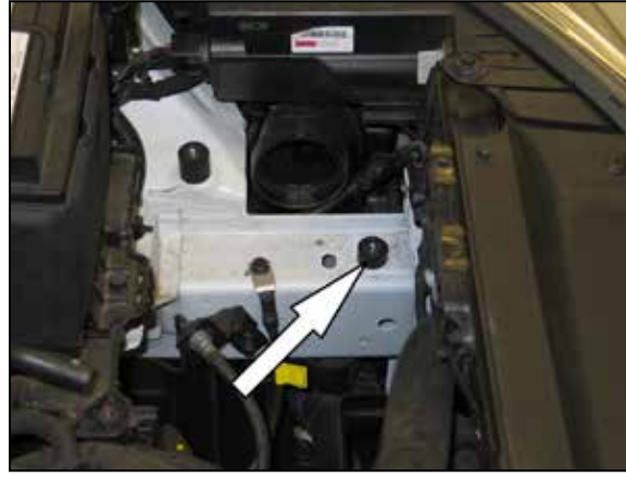
12. Install the 1/2" rubber mounted stud into the front factory air box mounting location as shown.
