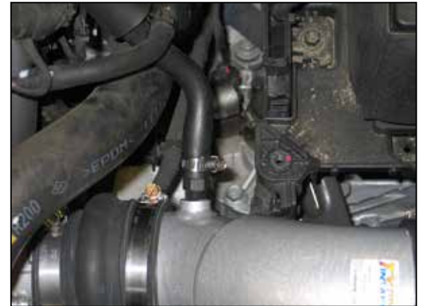
21. Reroute the crank case vent line under the fuel line and then install it onto the crank case vent fitting on the intake tube. Secure with the provided hose clamp.
