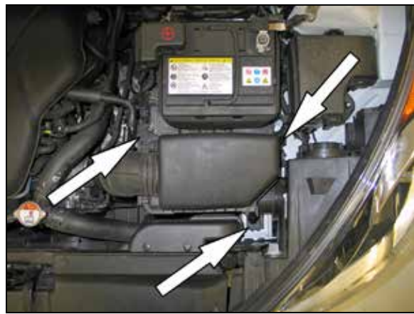
4. Remove the three bolts securing the factory air box assembly onto the inner fender.
