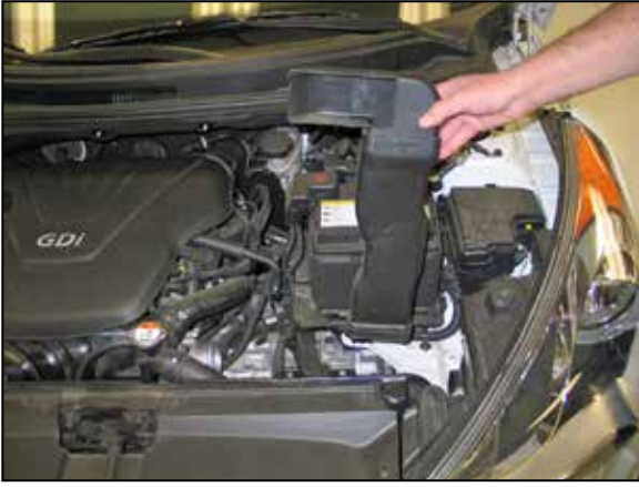
7. Remove the fresh air intake duct.
