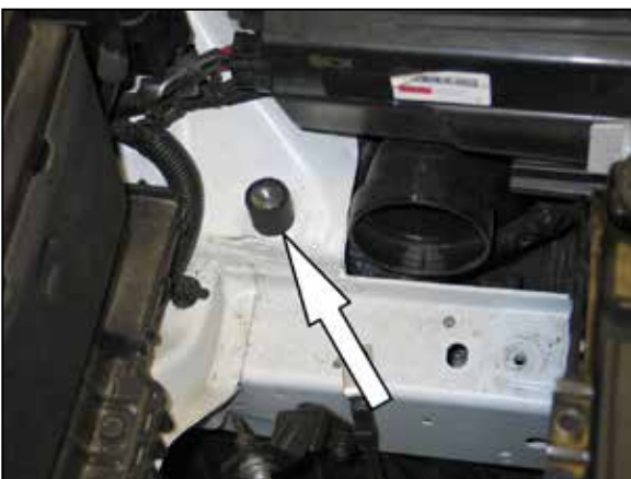
11. Install the 1" rubber mounted stud into the rear factory air box mounting location as shown.
