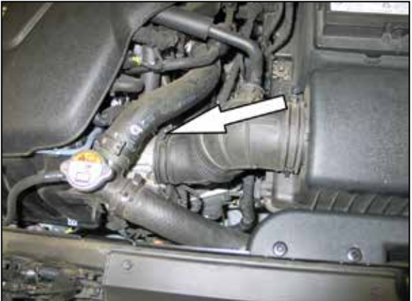
2. Loosen the hose clamp securing the intake tube to the throttle body.
