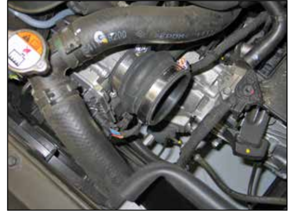
17. Install the provided silicone hump hose (5-574) onto the throttle body and secure with the provided hose clamp.
