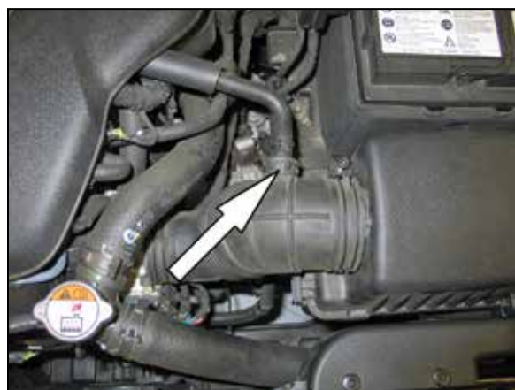
3. Disconnect the crank case vent hose from the factory intake tube.
