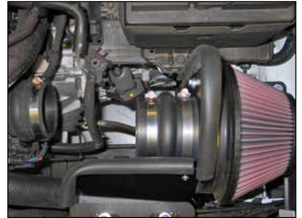
18. Install the provided silicone hump hose (5-576) onto the filter adapter and secure with the provided hose clamp.
