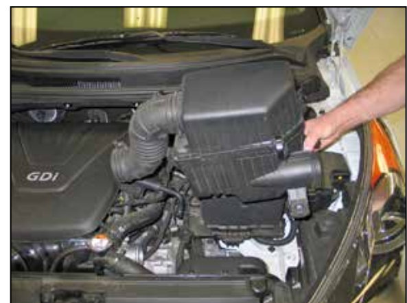
5. Remove the air box assembly from the vehicle. NOTE: K&N Engineering, Inc., recommends that customers do not discard factory air intake.
