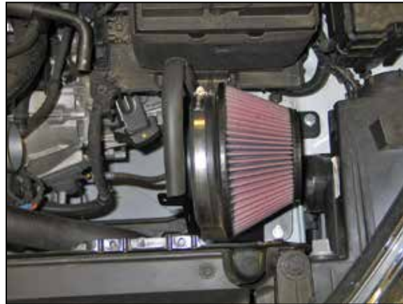
15. Install the filter assembly into the heat shield and secure with the rear mounting bolt provided only at this time.
