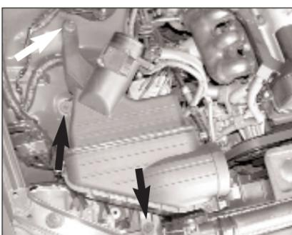
9. Remove the 3 bolts that retain the air box onto the vehicle.
