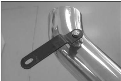
21. Secure the provided bracket to the K&N® intake tube using the provided hardware as shown.
