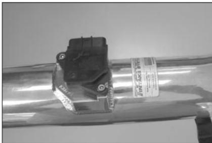
23. Install the mass air sensor into the K&N® intake tube using the provided hardware as shown.
