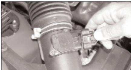
3. Disconnect the mass air electrical connection.
