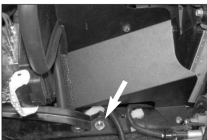
18. On 2002-2005 models slide the ABS pump bracket back to its original position and secure using the stock hardware as shown.
