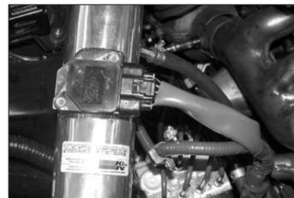
31. Reconnect the mass air sensor electrical connection as shown.
