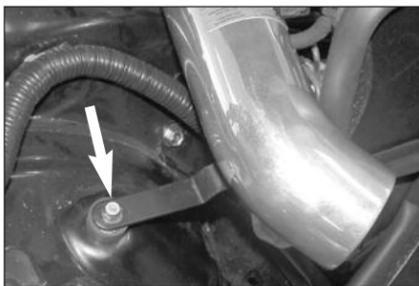
25. Secure the bracket to the rubber mounted stud using the provided hardware as shown.
