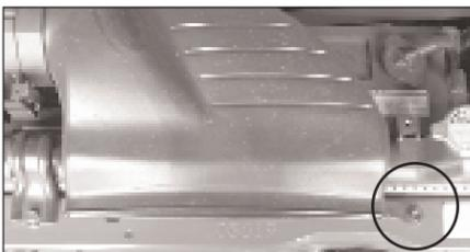
8. Loosen and remove the 10mm bolt that retains the fresh air intake to the vehicle then remove from the vehicle.
