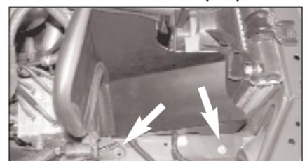
15. On 2001 models install the heat shield and secure using the provided hardware as shown.
