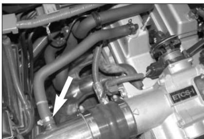
26. Remove the stock spring clamp and secure the crank case vent hose to the vent on the K&N® intake tube using the provided hose clamp as shown.
