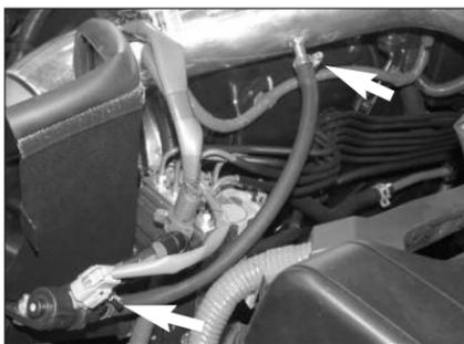
28. Connect the provided silicone hose to the evap solenoid, then, connect the other end to the vent on the K&N® intake tube with the provided hose clamps as shown.
