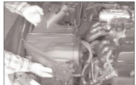
12. Remove the complete air box from vehicle. **NOTE: K&N Engineering, Inc., recommends that customers do not discard factory air intake.**
