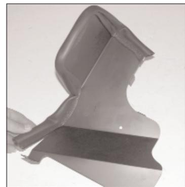
13. Install edge trim onto the heat shield as shown. Trim if needed.
