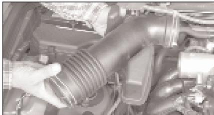
7. Remove the intake tube as shown.
