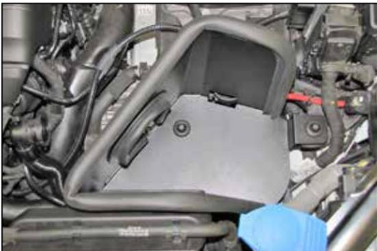
11. Install the heat shield assembly onto the factory air filter housing mounting studs.
