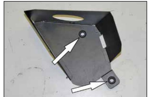
5. Install the two provided grommets into the heat shield as shown.
