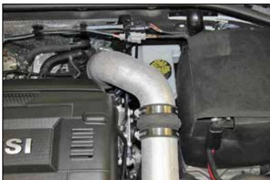
18. Install the rear K&N® intake tube into the coupling hose on the front intake tube and then into the coupling hose at the turbo inlet, adjust the tubes for best fit and then secure with the provided hose clamps.
