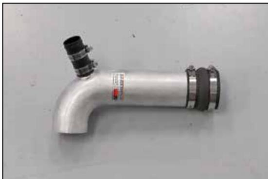
16. Install the remaining coupling hose (08185) onto the K&N® intake tube as shown.
