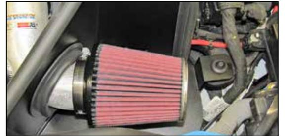
20. Install the K&N® air filter onto the intake tube and secure with the provided hose clamp.
