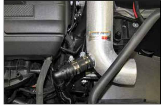
19. Connect the secondary air hose onto the Quick disconnect fitting and connect the vacuum line to the fitting installed into the K&N® intake tube.
