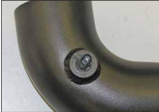
28. Install the inlet air temperature sensor into the K&N® intake tube as shown.
