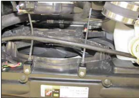
30. Install the tie wrap equipped brackets onto the factory intake tube mounting locations on the fan shroud using the provided hardware. Then secure the coolant over flow hose with the tie wraps.
