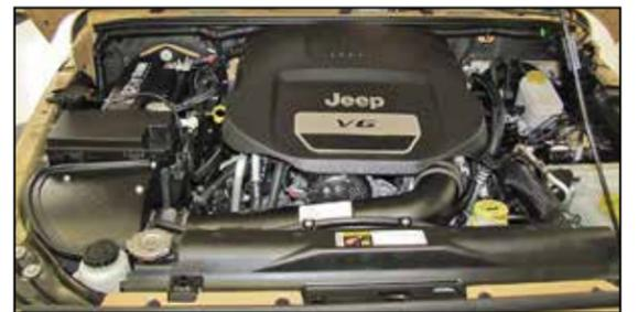
34. Reconnect the vehicle's negative battery cable. Double check to make sure everything is tight and properly positioned before starting the vehicle.
