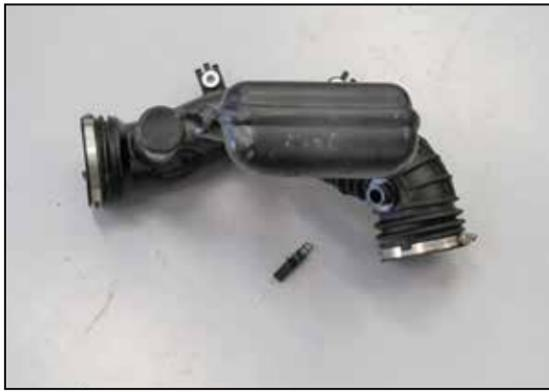
27. Remove the inlet air temperature sensor from the factory intake plenum as shown.
