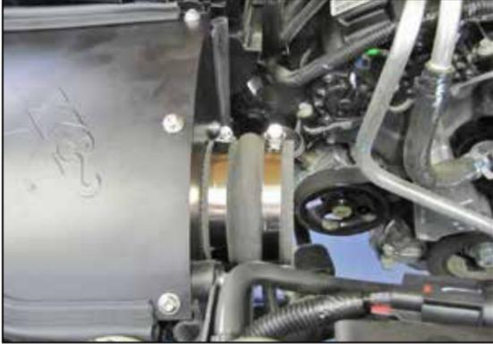
23. Install the provided hump hose (08699) onto the filter adapter and secure with the provided hose clamp.
