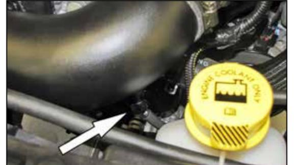
33. Reconnect the inlet air temperature sensor electrical connection and then reinstall the engine cover.
