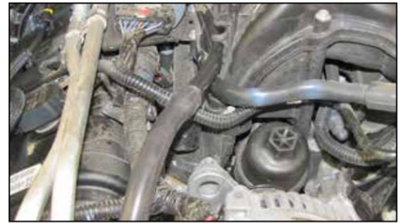
32. Connect the open end of the crank case vent hose to the factory crank case vent tube as shown.
