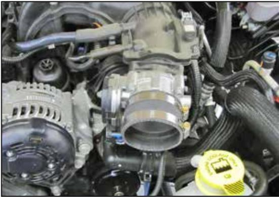
24. Install the provided silicone hose (08690) onto the throttle body and secure with the provided hose clamp.
