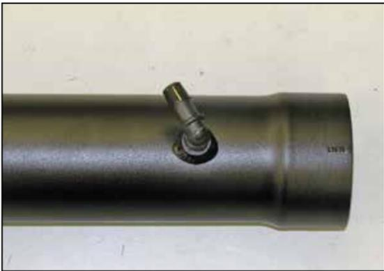
25. Install the 90°, 1/2" vent fitting into the K&N® intake tube as shown.
