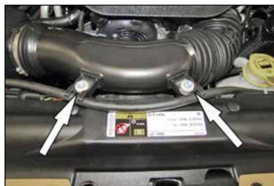
3. Remove the two bolts which secure the factory intake tube to the fan shroud.
