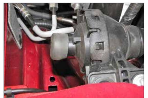
6. Install the provided cap onto the drum as shown.
