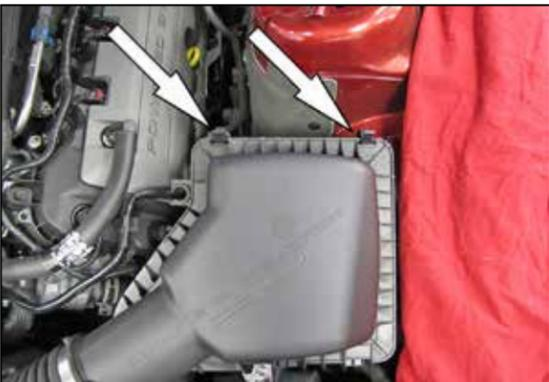
10. Release the two upper air box retaining clips and then remove the upper air box and intake tube from the vehicle.
