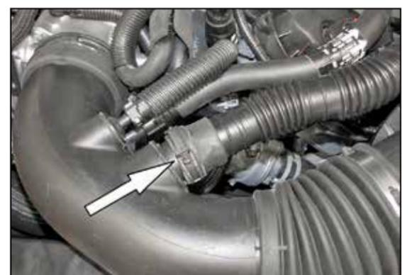
5. Release the clamp that secures the pulse hose to the intake tube and then remove the pulse hose from the vehicle.
