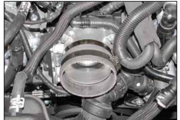
18. Install the provided silicone hose (08698) onto the throttle body and secure with the provided hose clamp.
