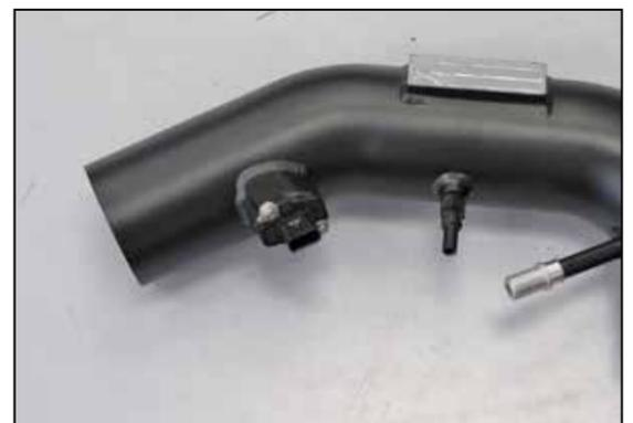
21. Install the mass air sensor into the K&N® intake tube and secure with the provided hardware.
