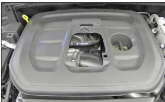
2. Lift up the inspection cover and remove the bolt that secures the decorative engine cover. Then remove the decorative engine cover from the vehicle.
