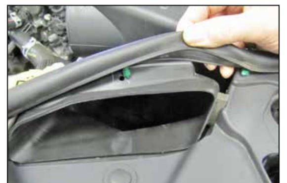
6. Unhook the hood seal mounting pin from the fresh air intake scoop.
