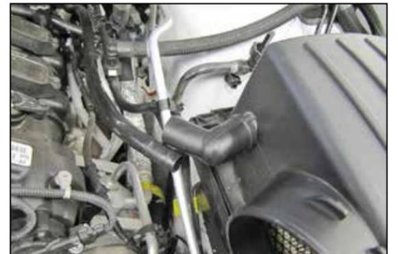
5. Disconnect the crank case vent tube from the elbow attached to the factory air filter housing as shown.
