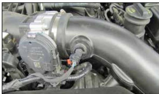
3. Disconnect the inlet air temperature sensor electrical connection.
