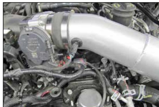
20. Reconnect the inlet air temperature sensor electrical connection.
