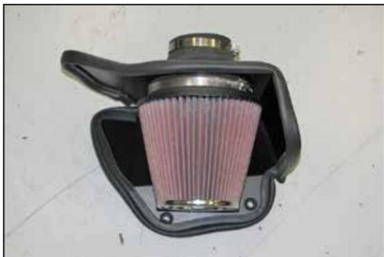
13. Install the K&N® air filter onto the filter adapter and secure with the provided hose clamp.
