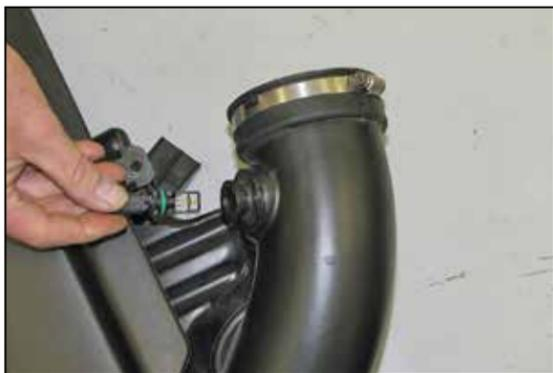
15. Remove the inlet air temperature sensor from the factory intake tube.
