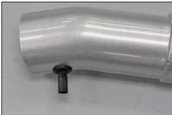
16. Install the provided grommet into the K&N® intake tube then remove the O-Ring from the inlet air temperature sensor and then install the sensor into the grommet install into the K&N® intake tube.
