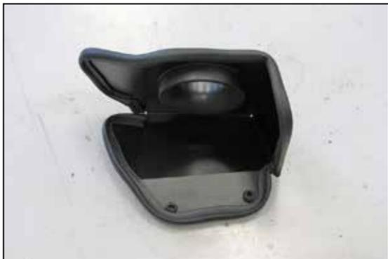
11. Install the provided edge trim onto the heat shield as shown.
