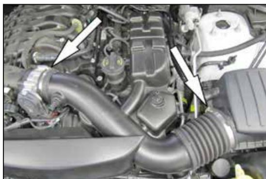
4. Loosen the hose clamps securing the intake tube to the throttle body and air filter housing and then remove the intake tube assembly from the vehicle.
