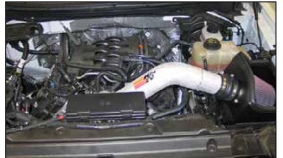
23. Reconnect the vehicle's negative battery cable. Double check to make sure everything is tight and properly positioned before starting the vehicle.
