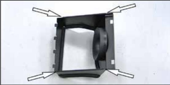
10. Install the two 9" sections of edge trim onto the bottom of the heat shield as shown.
