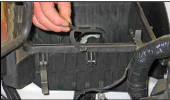
12. Remove the center airbox retaining clip.
