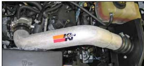
19. Install the K&N® intake tube assembly into the silicone hose attached to the filter adapter and then into the silicone hose on the throttle body. Secure with the provided hose clamps.
