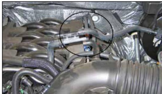
4. Disconnect the EVAP hose from the check valve as shown.
