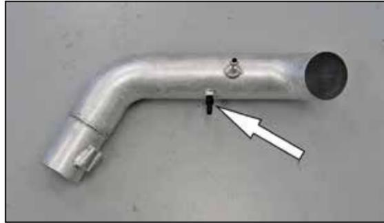
16. Install the provided 3/8" hose fitting into the K&N® intake tube as shown.
