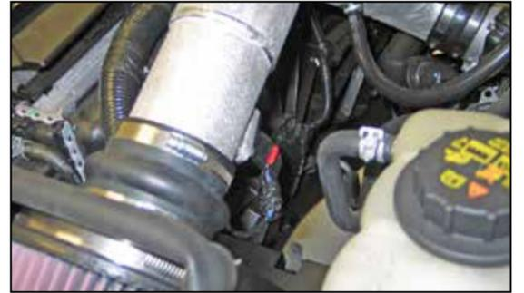
22. Reconnect the mass air sensor electrical connection.
