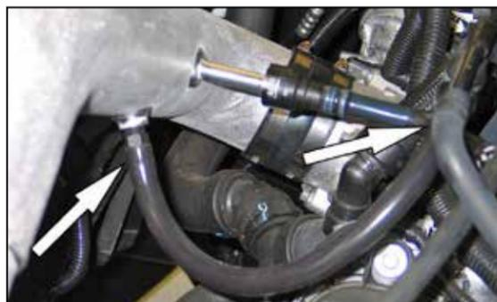
21. Install the provided silicone hose onto the 3/8" hose fitting installed in the K&N® intake tube; attach the open end to the EVAP check valve.
