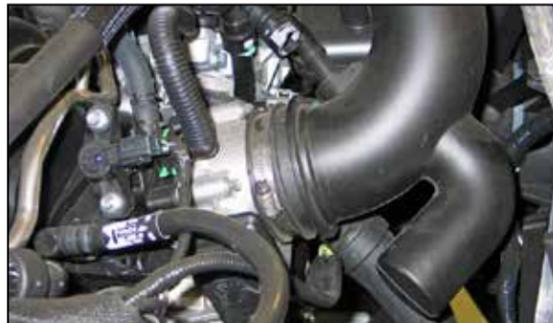
5. Loosen the hose clamp securing the factory intake tube to the throttle body.
