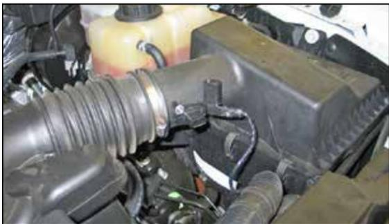
2. Release the red locking tab and then disconnect the mass air sensor electrical connection.
