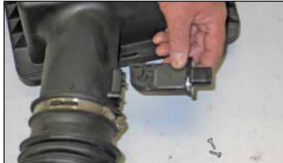
17. Remove the two screws securing the mass air sensor, then remove from the stock intake tube as shown.
