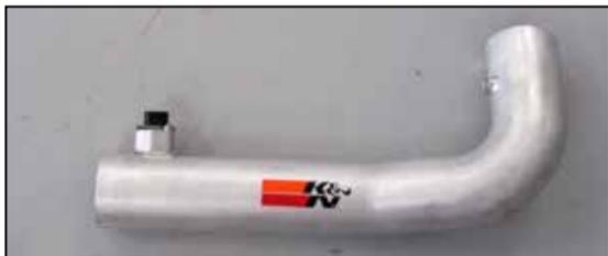
15. Install the mass air sensor assembly into the K&N® intake tube and secure with the provided hardware.
