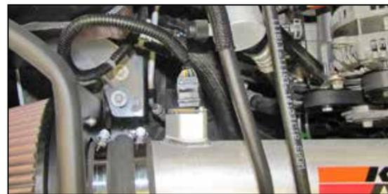
19. Reconnect the mass air sensor electrical connection.
