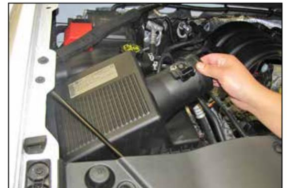
6. Lift up and remove the air filter housing from the vehicle.
