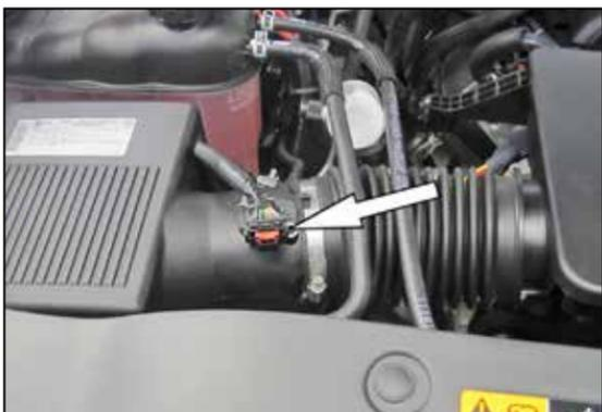
2. Disconnect the mass air sensor electrical connection and unhook the wiring harness from the air filter housing.
