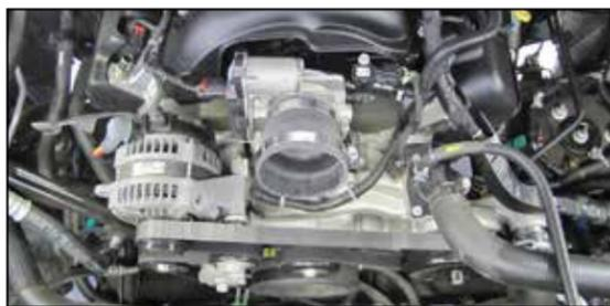
12. Install the provided step hose (084055) onto the throttle body and secure with the provided hose clamp.
