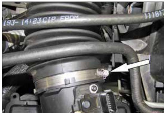
4. Loosen the hose clamp securing the intake tube to the air filter housing.
