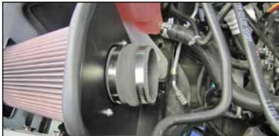
13. Install the provided hump hose (08699) onto the filter adapter and secure with the provided hose clamp.
