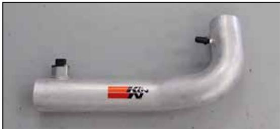
16. Install the vent fitting into the K&N® intake tube. **NOTE: Plastic NPT fittings are easy to cross thread. Install the vent fitting "hand" tight, then turn it two complete turns with a wrench.**
