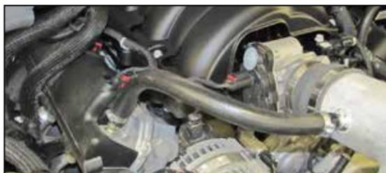
18. Install the provided crank case vent hose onto the valve cover port and onto the vent installed into the intake tube. Secure the hose with the provided hose clamps.
