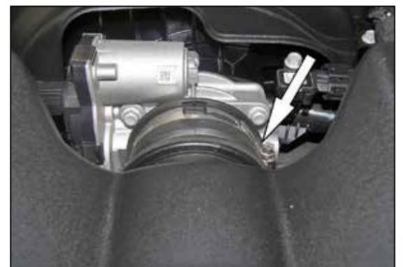
5. Loosen the hose clamp securing the intake plenum to the throttle body and then remove the intake plenum from the vehicle.
