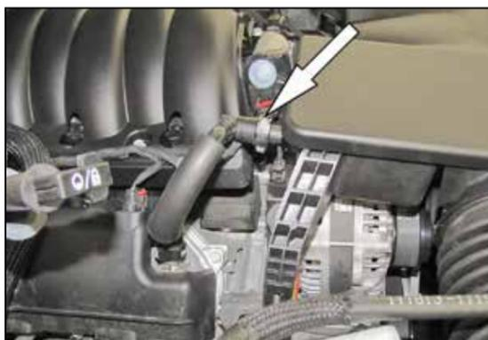
3. Disconnect the crank case vent from the intake plenum and valve cover port and remove it from the engine.
