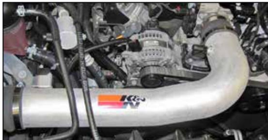
17. Install the K&N® intake tube into the hose at the filter adapter and then into the hose at the throttle body. Adjust the tube for best fit and then secure with the provided hose clamps.
