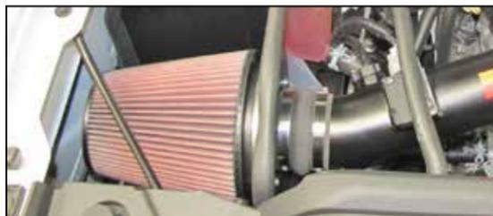
19. Install the K&N air filter and secure with the provided hose clamp.
