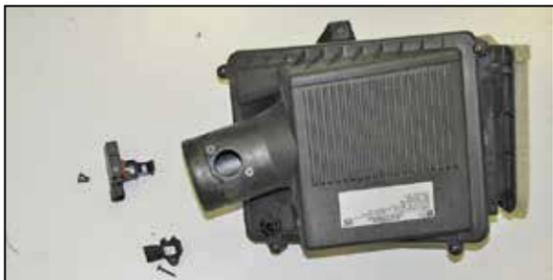
12. Remove the screws securing the mass air sensor and humidity sensors into the air filter housing and then remove the sensors.
