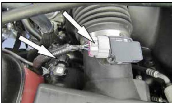
3. Disconnect the mass air sensor and humidity sensor electrical connections.
