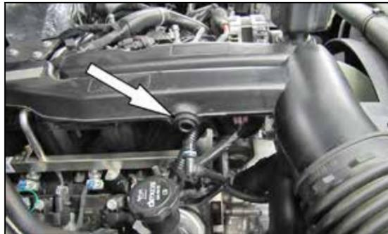
4. Disconnect the crank case vent hose from the intake tube plenum as shown.
