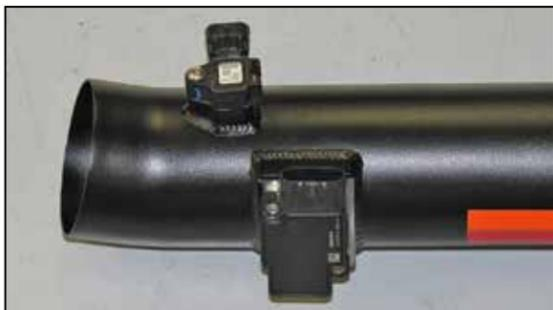
13. Install the mass air sensor and humidity sensors into the K&N intake tube and secure with the provided hardware.
