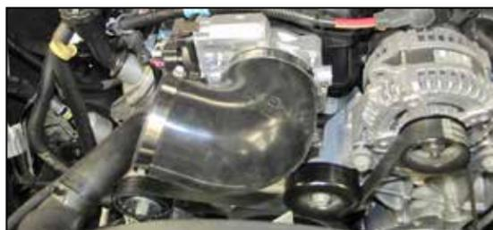
16. Install the provided coupler hose (084086) onto the throttle body but do not completely tighten at this time.
