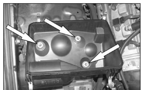
6. Remove the air box lid and filter to gain access to the three bolts that retain the air box to vehicle.
