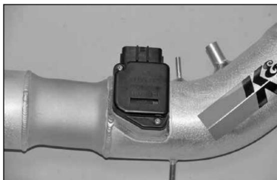
15. Install the mass air sensor into the K&N® intake tube and secure with the provided bolts as shown.
