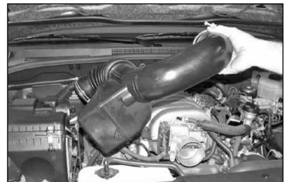
5. Loosen the hose clamp at the throttle body and air box, then remove intake tube from vehicle.
