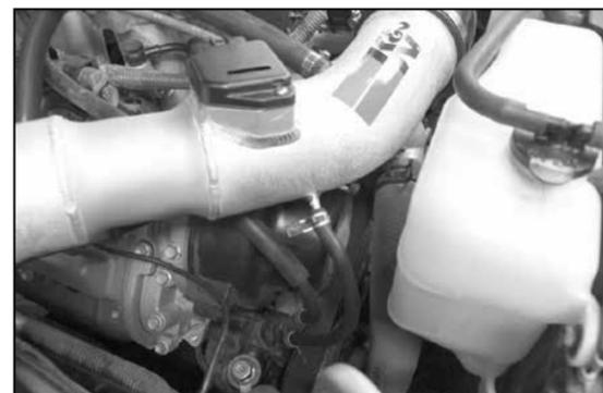
19. Connect the factory power steering pressure switch vent hose onto the K&N® intake tube as shown.
