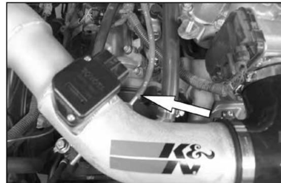
18. Connect the factory fuel pressure vent hose onto the K&N® intake tube as shown.
