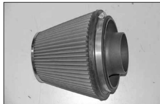
20. Install the filter adapter into the air filter as shown and secure with the provided hose clamp.
