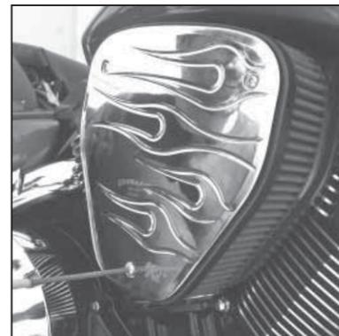
27. Install the front plate on the K&N® air filter
