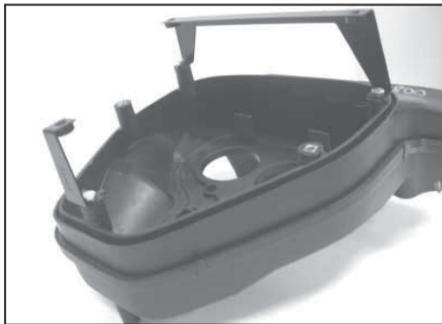
20. Using the supplied Hex bolts, install the large and small brackets onto the air cleaner housing.
