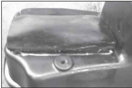
18. Install the large plug into the air cleaner housing.
