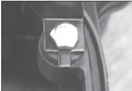
21. Make sure that a flat side of the Hex bolt is even with the tab on the bracket.
