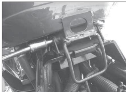
4. Remove the fuel tank hinge bolt.
