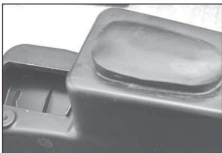
16. Install the small plug into the air cleaner housing.
