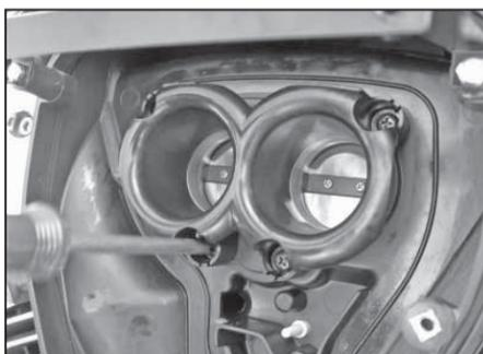
24. Reinstall the air funnel and tighten the screws.
