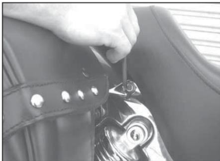
1. Remove the seat bolts (one on each side)
