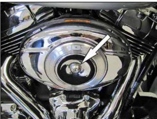
2. Remove the bolt securing the bonnet to the air filter and then remove the bonnet from the air filter.
