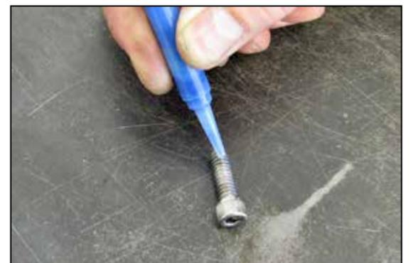
7. Apply one drop of the provided thread locker to the provided throttle body bolts.
