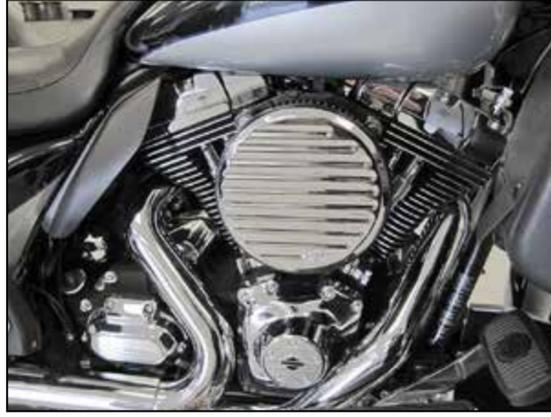
13. Install the K&N® air filter and front plate onto the back plate and secure with the provided hardware. **NOTE: It may be helpful to use a small screwdriver to position the filter into the grooves of the front and back plate while tightening the hardware.**
