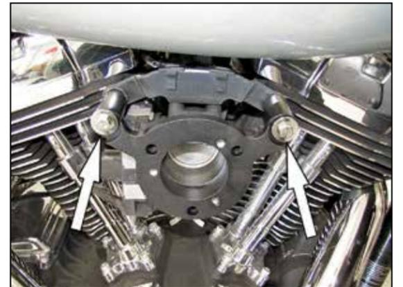
6. Install the K&N® adapter onto the engine and throttle body using the provided breather bolt.
