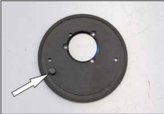
9. Install the provided rubber plug into the back plate from the back side as shown.
